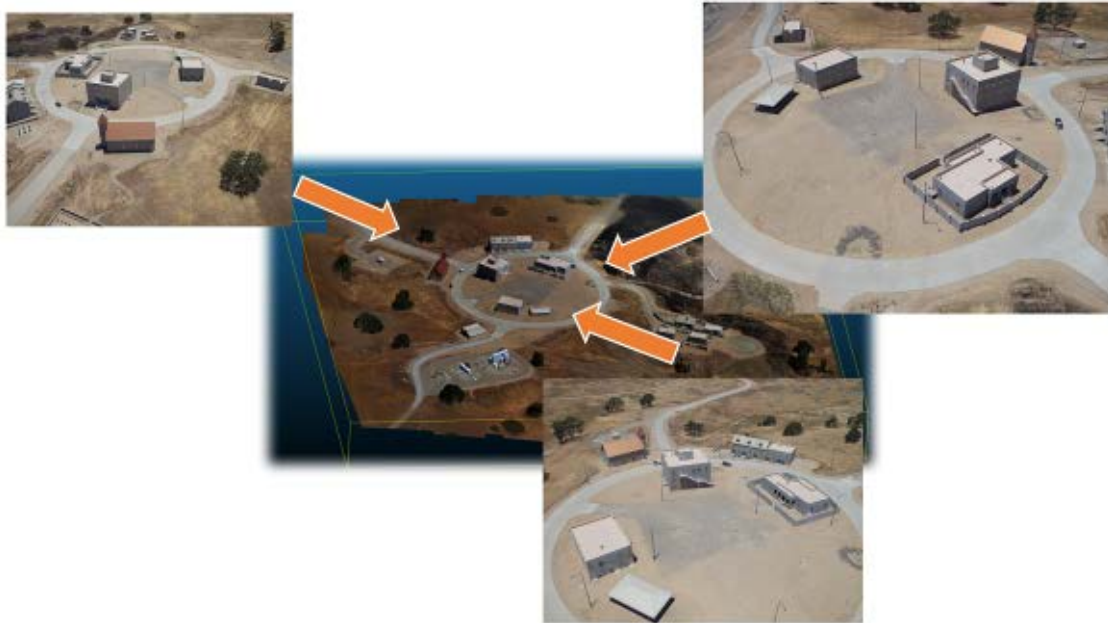
Figure 30. Development of point cloud based on multiple images from various orientations
