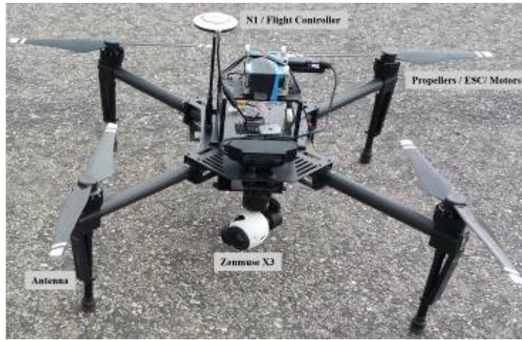
Figure 58. Overview of Matrice 100
