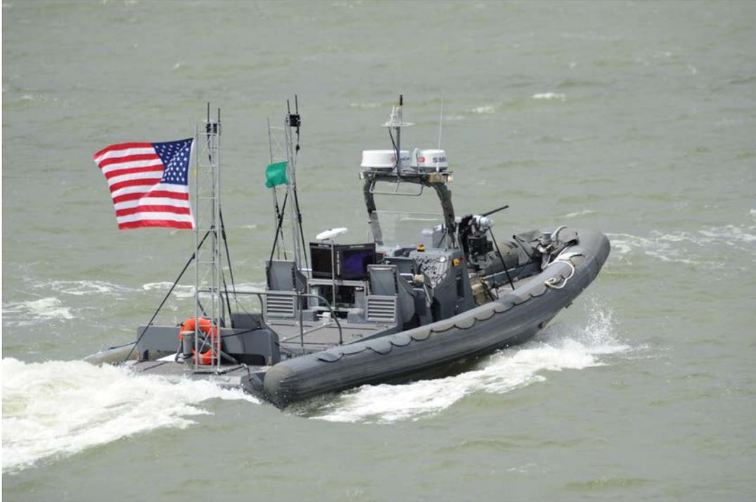
Figure 3. RHIB USV Equipped with CARACaS.
