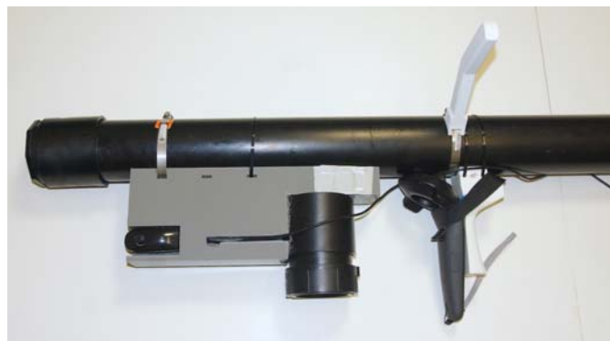
Figure 55. Trigger switch fixed inside housing with slit for cable adjustment
