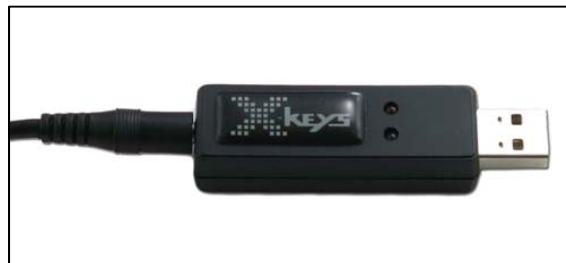
Figure 41. USB adapter for trigger switch device. Source: Fentek Industries (n.d.).
