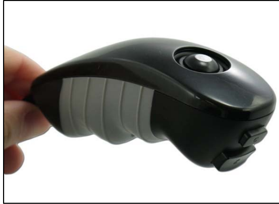
Figure 40. Trigger switch device containing three buttons. Source: Fentek Industries (n.d.).
