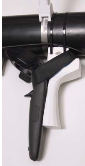
Figure 54. Trigger assembly and optical sight prop attached to main tube using metal clamps and plastic tie wraps
