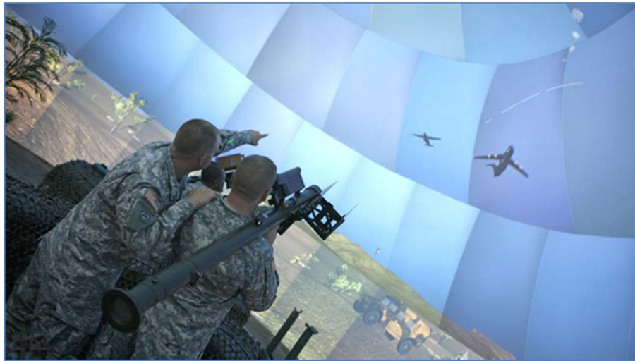
Figure 2. IMTS with dome projection for immersive display. Source: Weirauch (2013).
