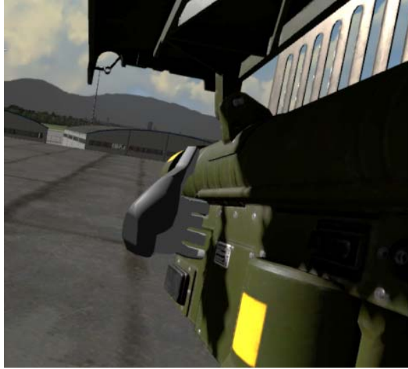
Figure 60. Hand tracking by Leap Motion and wrongly positioned virtual hand in VE
