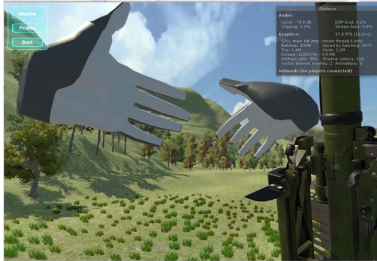
Figure 46. Virtual hands depiction in the VE as detected by the Leap Motion controller
