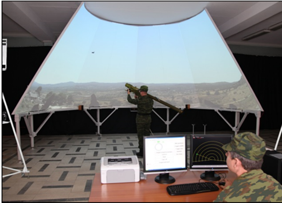
Conical projection display with 192-degree horizontal FOV.
