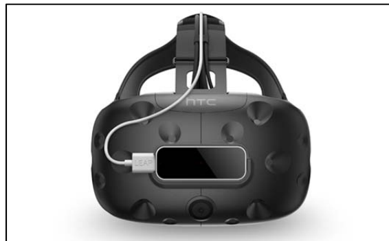
Figure 22. Leap Motion sensor installed on HTC Vive headset. Source: Leap Motion (n.d.).
