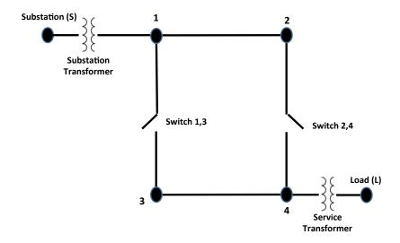
The Basic Test Circuit With Cycle consists of a substation with functionally infinite capacity and a moderate load, each with their own transformer. Between them is a cycle of four nodes, with two of the four edges containing switches. Unlike the Basic Test Circuit, there is no shunt capacitor at the load.
