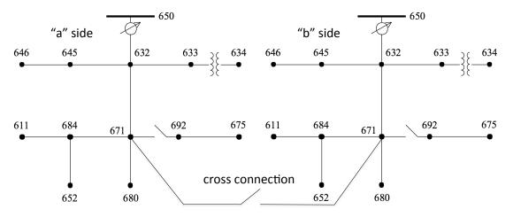
The duplicated 13 node test feeder with "a" and "b" sides, connected by a line between nodes 671a and 671b. Electrical parameters for both sides are the same as the original IEEE 13 node test feeder, described in Tables 4.1 and 4.2. The cross connection line is 3-phase with  $R_{ij}$  and  $X_{ij}$  values copied from line 692-675. The  $T_{ij}$  value is very low at 15 amps.
