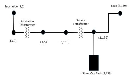
The Basic Test Circuit consists of a substation with functionally infinite capacity, a transformer, connective line leading to a service transformer, and a commercial grade customer with moderate loading and a shunt capacitor bank. When operated, no load should be shed in this test network.
