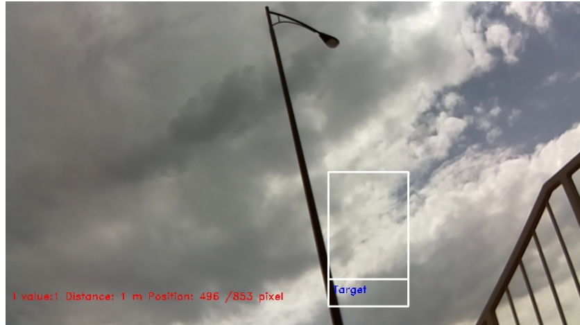
Figure 71. A Cloudy Condition Caused False Positive when Camera Was Pointing Upward
