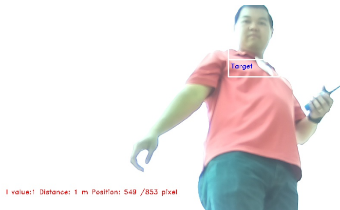
Figure 70. Facial Image Detection Capability of the WGS Node under Highly Exposed Lighting Condition
