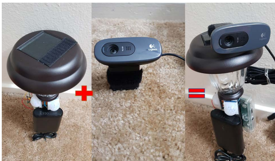
Figure 40. Mounting of USB Webcam onto the Solar Garden Light for Variant A of WGS Node
