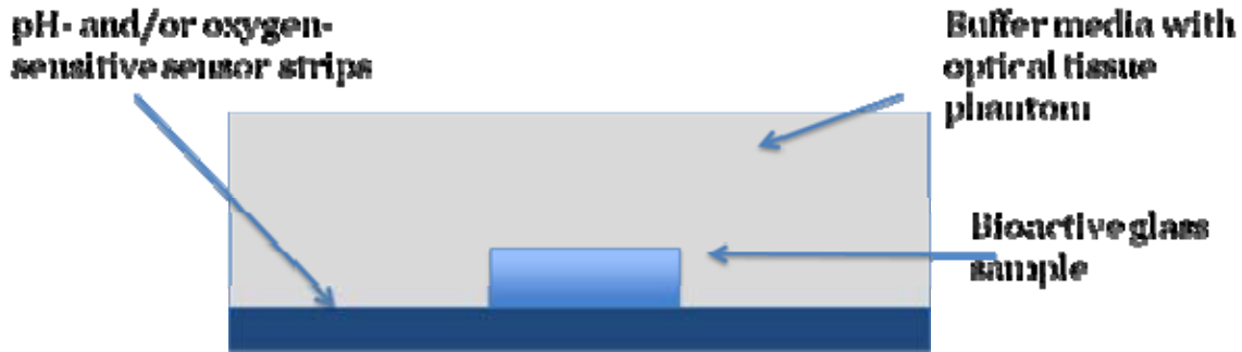
Fig. 33. Bioglass conversion test environment. Fluorescent sensing strips/films that are sensitive to oxygen concentrations or pH are mounted on substrate. Illumination by blue light from above leads to fluorescence and collection of the image through a standard CMOS or CCD camera. (Henthorn and Kim, Missouri S&T).
