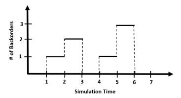
This simplified image demonstrates the concept of a time varying statistic. When we calculate EBO, we are interested in both the volume of backorders and how long they go unfilled to calculate the average backorder level. To calculate the EBO for this small example, we sum the area under the curve (7) and divide by the total simulated time (7) and return an EBO of 1.
