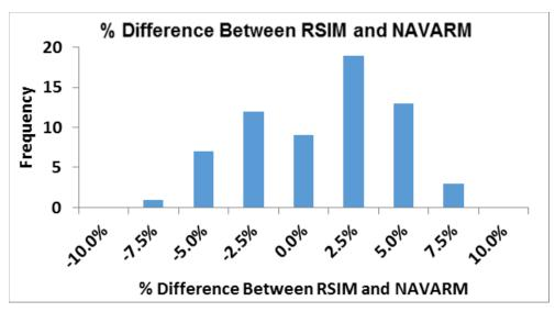
This figure shows the summary histogram of the differences in expected availability between RSIM and NAVARM for the 64 WS types tested. Out of the 64 WS types analyzed, 53 have expected readiness levels within 5% and the mean difference for all WS types in this sample is .2% with no systemic bias to over or under estimate readiness noted.
