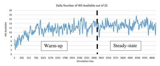
To ensure a bias is not introduced in the RSIM output from starting condition levels, a truncation point is selected that will allow the system to reach a steady-state before data collection begins. Here we depict daily readiness levels for a WS type with 22 individual WS and employ a 10-day running average of available WS to make the trend more apparent. This WS arrives at steady-state between 1,000 and 3,000 simulated days. We select a conservative truncation point of 3,000.
