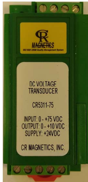
Figure 21 CR Magnetix CR5311-75 DC Voltage Transducer
