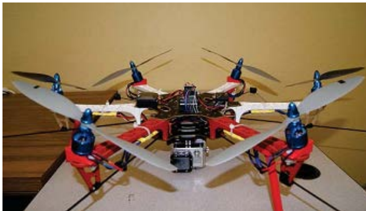
Figure 10. Hexacopter with Canted Propellers. Source: [29].
