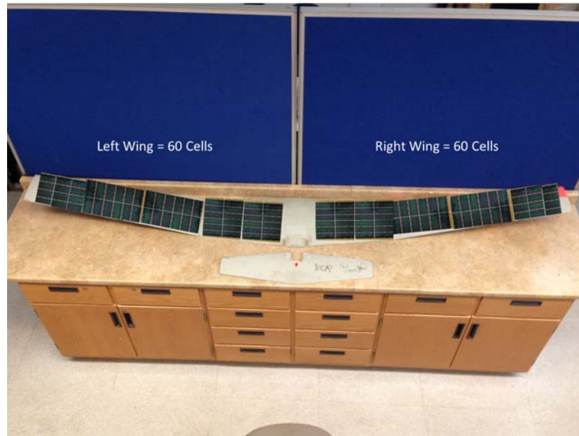
Figure 32. Conceptual Layout of Two Large Solar Panels on Puma Wing.
