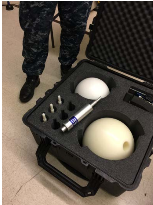
12” and 10” polyethylene spheres with LiI(Eu) detector in transport housing. Three additional polyethylene simulation detectors are also present.
