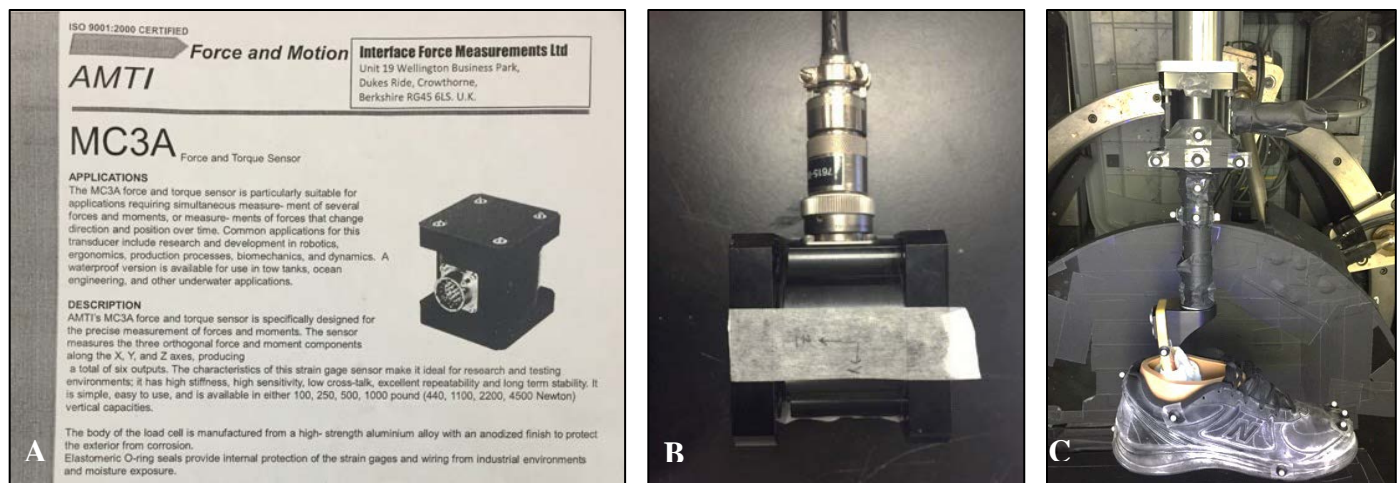
Figure 2: (A) AMTI 6-axis load cell added to RGS set-up for mechanical testing of prosthetic feet for improved accuracy of ankle torque data collection; (B) load cell unit separate from RGS mount; (C) load cell configured in-line with prosthetic pylon during data collection (aerial view of RGS).
