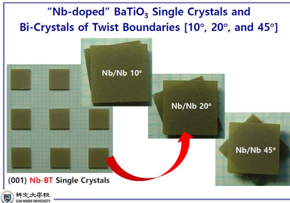
Fig. 33. Making twist boundaries by diffusion bonding of two "same" single crystal plates with specific misorientation angles
