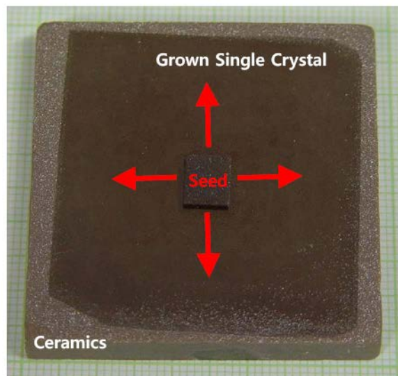
Fig. 6. SSCG of a \text{BaTiO}_3 single crystal in a polycrystalline precursor. by Ceracomp
