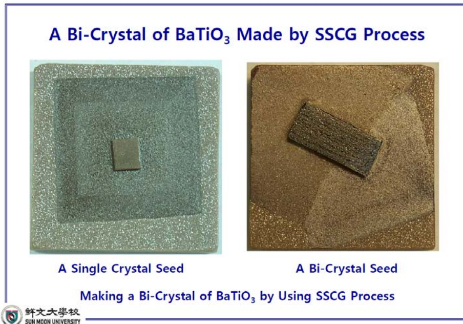
Fig. 31. Solid-state crystal growth of (a) one single crystal seed and (b) one bi-crystal seed: One large bi-crystal can be grown from one small bi-crystal by SSCG process.
