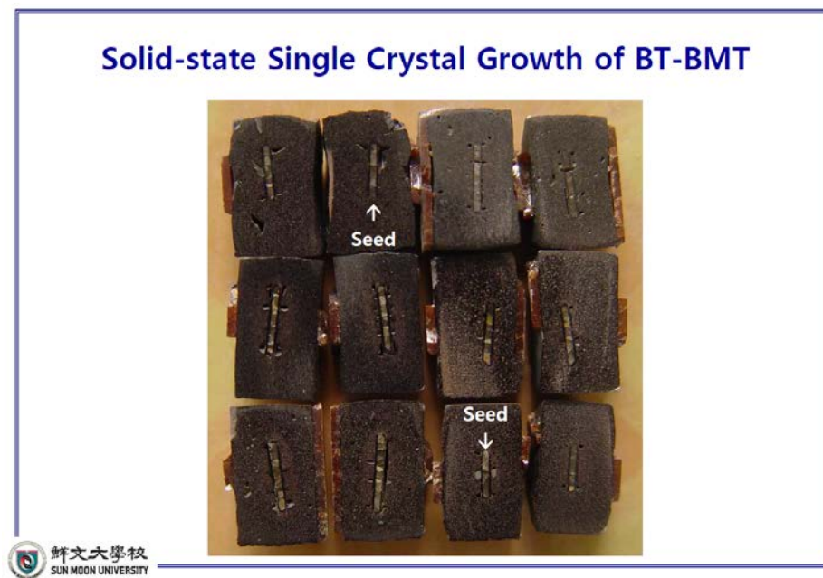
Fig. 30. Single crystal growth of BT-BMT from a \text{BaTiO}_3 single crystal seed inside BT-BMT ceramics
