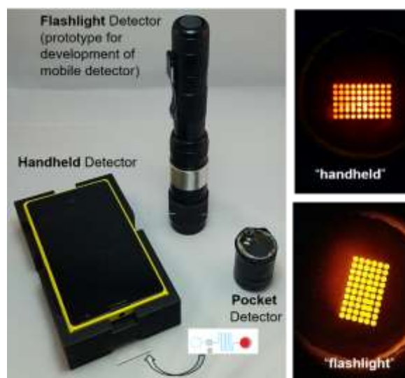
Fig. 4: Ruggedized portable detector with redundancy in design. Handheld, flashlight, and pocket embodiments shown. Representative array images with handheld and flashlight designs shown.
