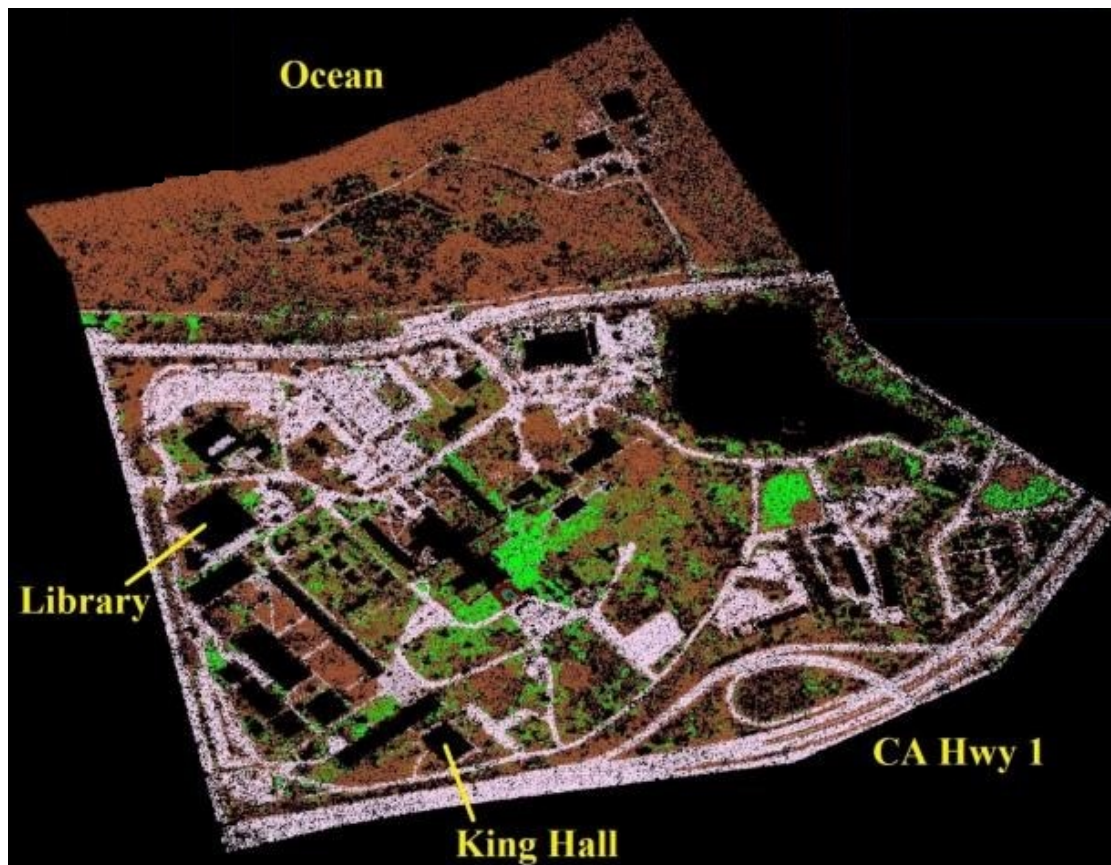
Figure 66. Ground Points Only in XYZ Space, Post-Spectral Subclassification.
