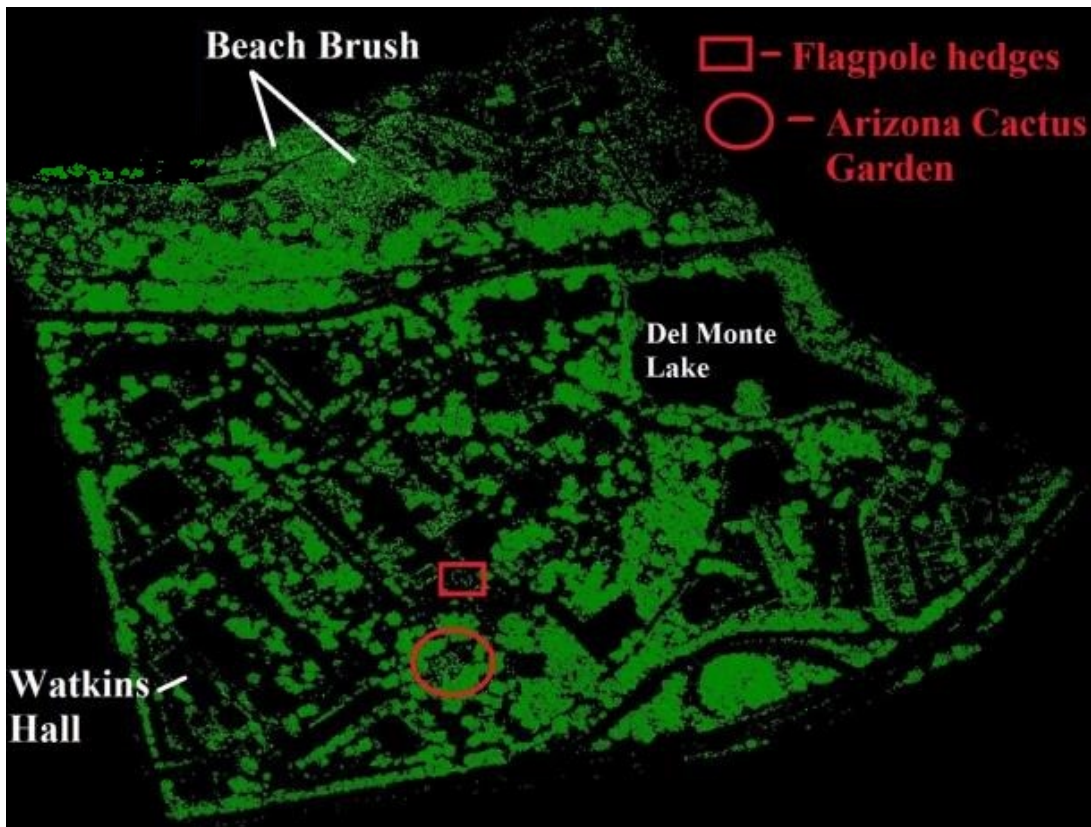
Figure 68. Vegetation Points Only in XYZ Space, Post-Spectral Subclassification.
