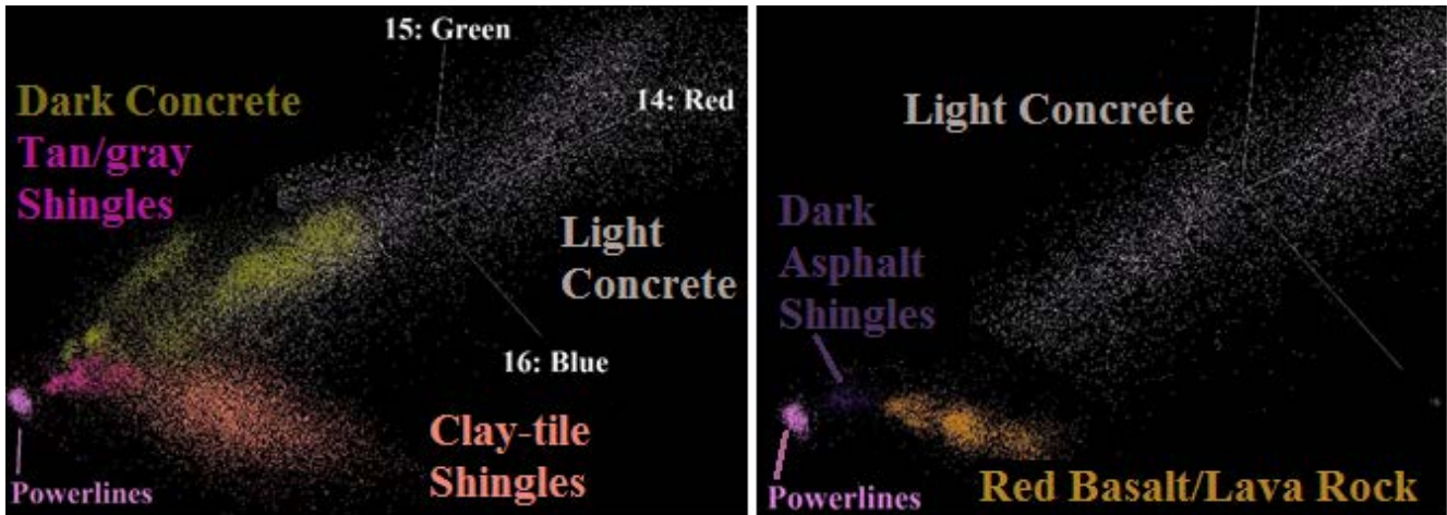
Figure 70. New Building Clusters in N-D VIS, Less the General Building Subclass.
