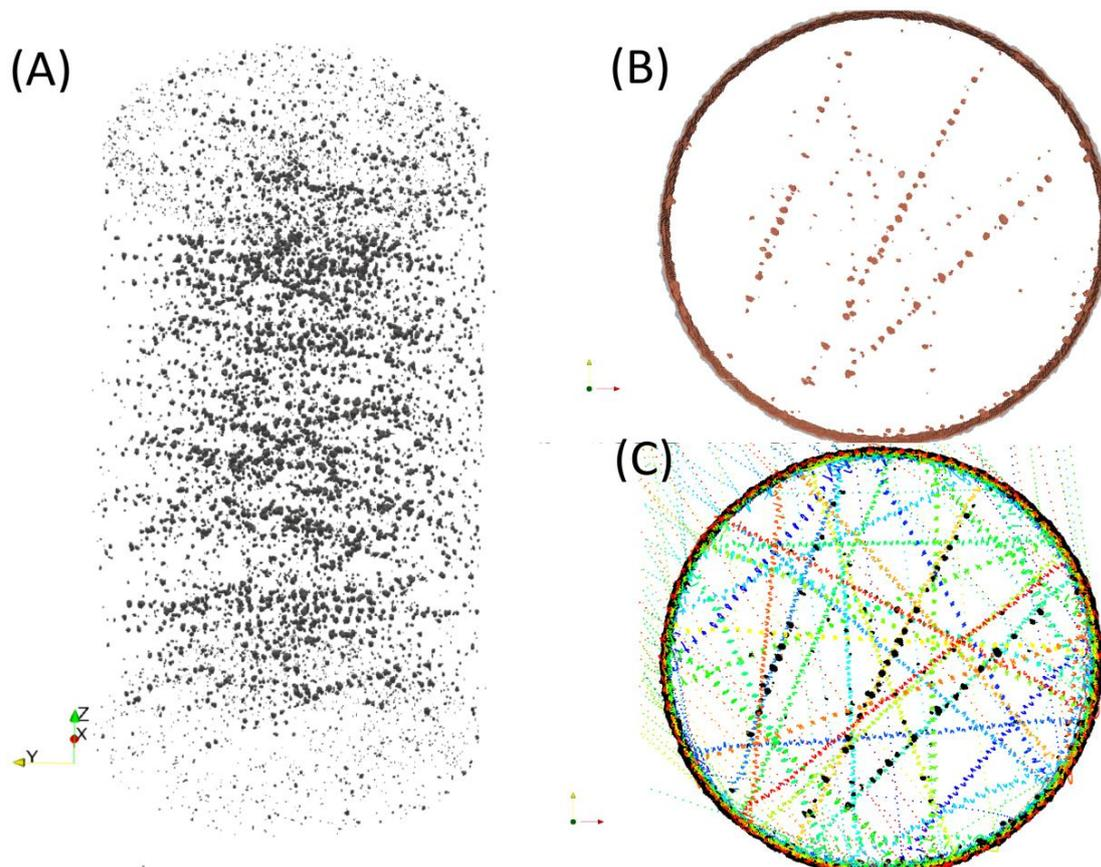
**Figure 6.** (A) Threshold reconstruction of CT scan of 10mm diameter, 20 mm tall cylindrical sample showing the internal porosity in the sample, (B) 1mm thick sub-region taken from the central portion of the cylinder showing the voids arranged in linear arrays, and (C) Overlay of the voids from (B) and the internal ‘stripe boundaries’ on the printed layers in that sub-region. Note the linear arrays lay on boundaries, but not all boundaries align with arrays of voids.
