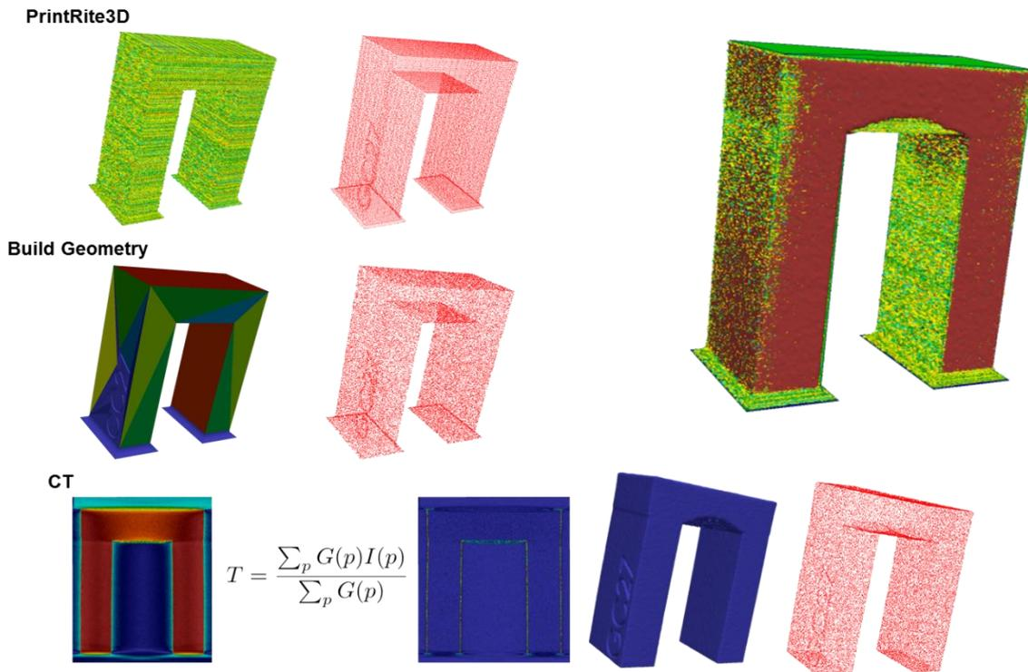
**Figure 3.** Data streams from CAD, CT and PrintRite3D, with point representation of sample surface. Larger inset shows final registry of full PrintRite3D data (green and yellow points) overlaid with threshold CT data (maroon surface) and CAD surface mesh (green triangles with blue edges on top surface). Note the point representations of the sample surface in the individual datasets are in their own reference frame and do not illustrate the magnitude of initial disregistry.
