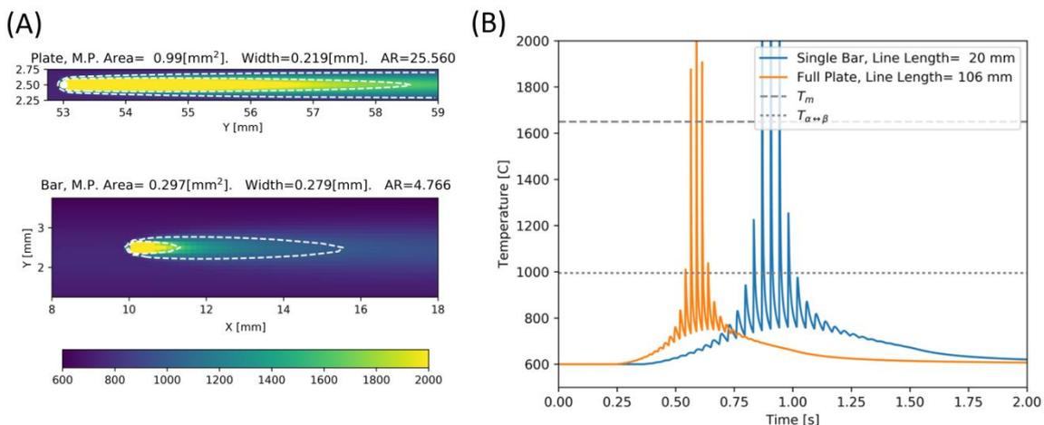
**Figure 12.** (A) Spatially-resolved thermal fields for a representative layer in the EBM build for the HED (bottom) and LED (top) regions, as calculated by the thermal model and (B) Time-temperature plots for a single point in the HED (blue) and LED (orange) regions. Note the differences in time above the melting temperature and the cooling rate across the beta transus.
