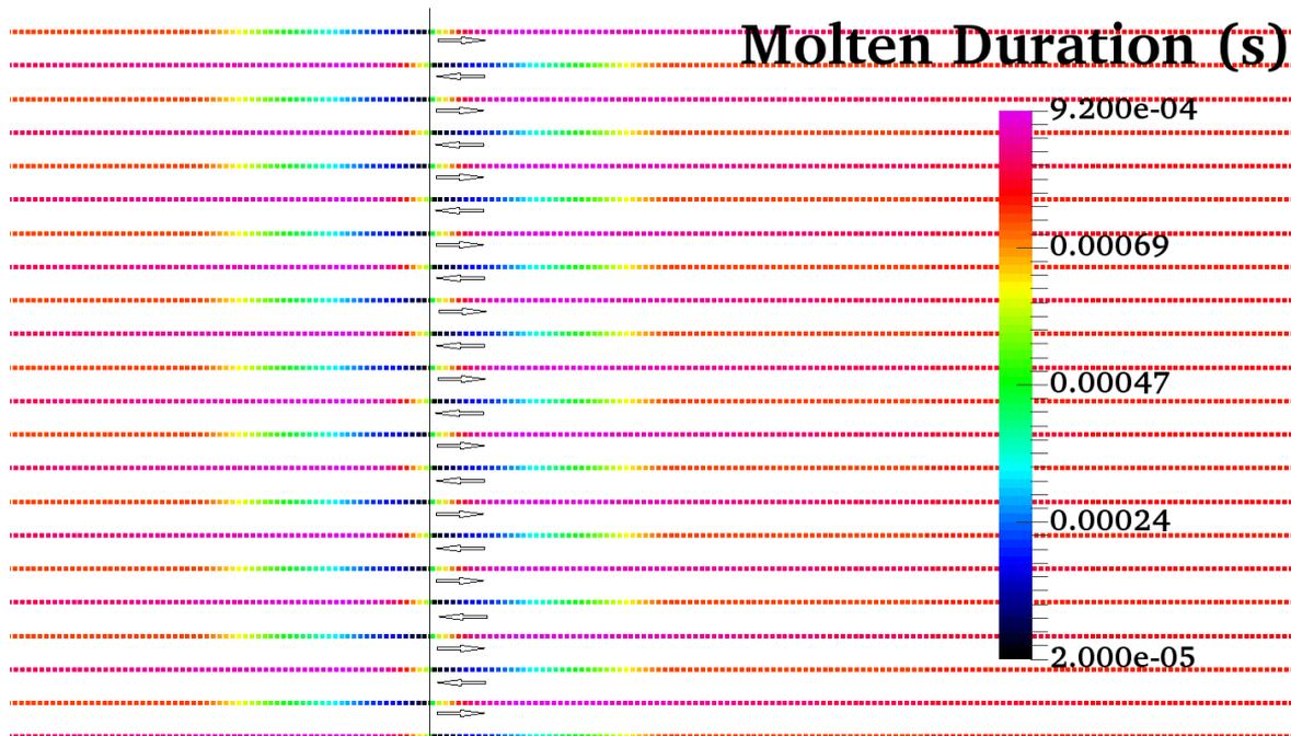
**Figure 9.** Discrete points along a set of scan vectors showing the time each point spent in the moving molten pool. The thin black line shows the position of the stripe boundary and the arrows show the direction of the beam into and out of the turn-around at the stripe boundary. The time spent molten decreases as the beam approaches the end of the track, leading to the ‘freezing in’ of a defect.
