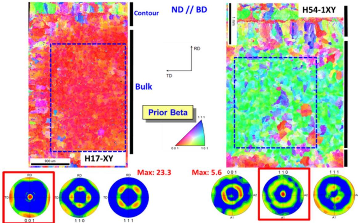
**Figure 11.** EBSD scans and pole figures for the HED (left) and LED (right) samples from the EBM build. The texture of the HED sample is ‘typical’ for EBM Ti-64, while the LED texture is ‘abnormal’. Note the build direction is normal to the plane of the scan.
