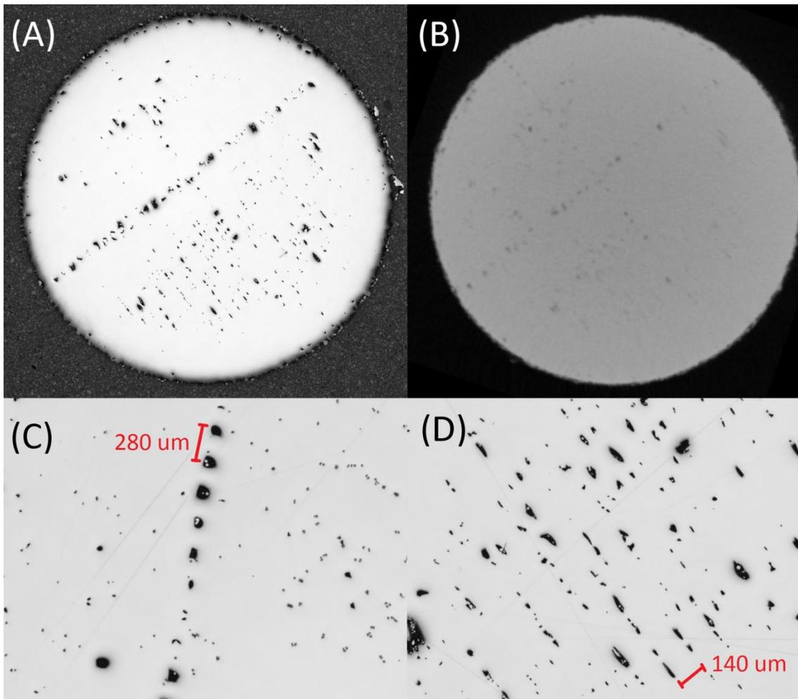
**Figure 7.** (A) High resolution optical microscopy montage showing the morphology of two populations of voids – montage covers the entire 10mm diameter of the part, (B) Section from CT reconstruction at same position as montage in (A), (C) Sub-image showing morphology of linear void arrays, and (D) Sub-image showing morphology of smaller, more elongated void population.
