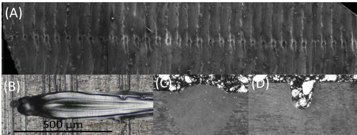
**Figure 8.** Images showing end-of-vector defects. (A) Top surface of sample from LPBF build, (B) Top view of single laser scan pass, (C) perpendicular section through track in (B) at midpoint along track, and (D) perpendicular section through track in (B) at endpoint where divot is present.
