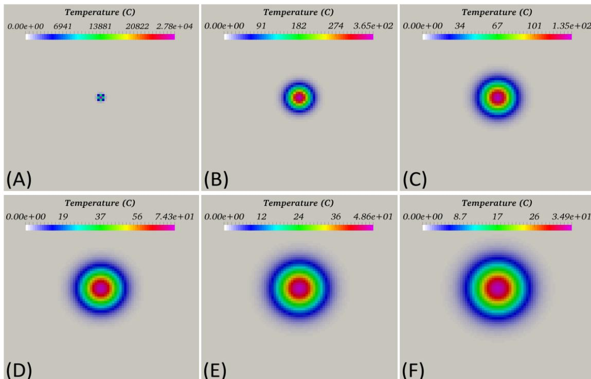
**Figure 4.** Sequence of time steps from the solution of a single discrete point source (A) 0.00002s, (B) 0.0002s, (C) 0.0004s, (D) 0.0006s, (E) 0.0008s, (F) 0.001s. Note the change in the temperature scale between time steps. (A) Illustrates the unrealistically high temperatures observed instantaneously after the source becomes active. Each panel has a 1mm x 1mm field-of-view.
