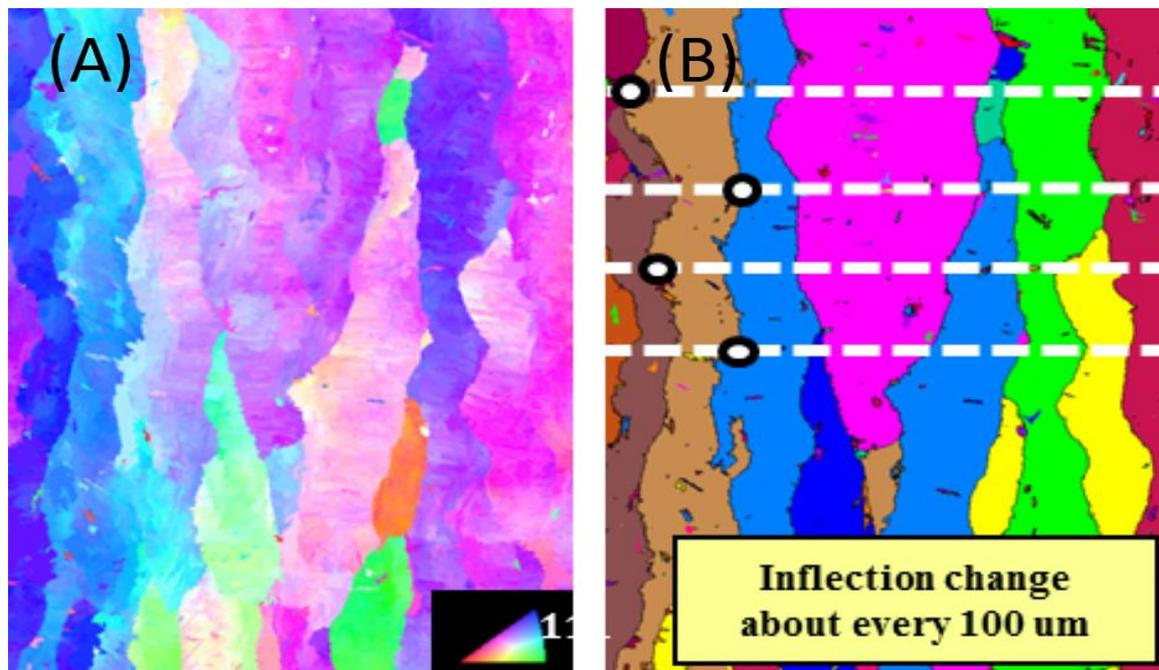
**Figure 13.** (A) EBSD scan of the LED sample perpendicular to build direction showing columnar features and (B) Prior beta grain reconstruction with annotations showing the serrated growth at roughly 30° to the build direction and inflections at multiples of the layer thickness (50µm), which is associated with the rotation strategy of the printing system.
