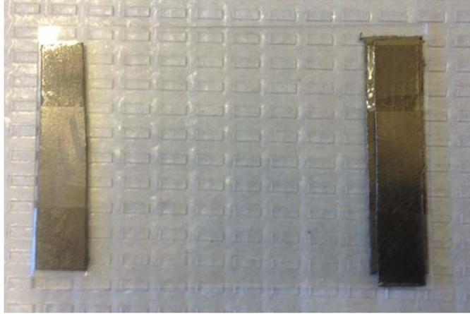
Figure 24. Microscope Slide with Grafoil Spacers Attached to the Edges
