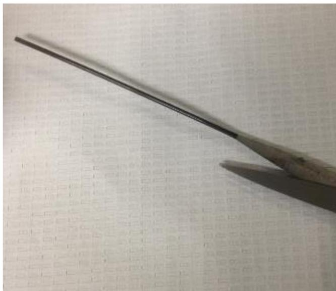
Figure 5. Stir Stick Modification Using Scissors
