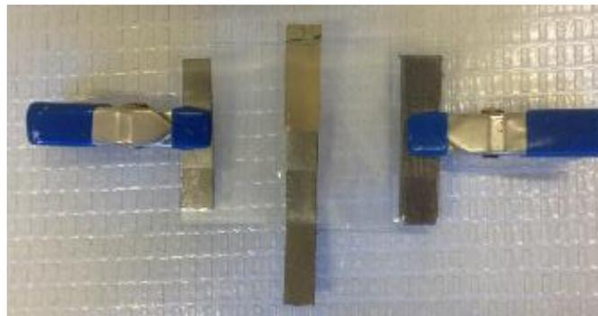
Figure 29. Second Spring Clamp Installed to Complete the Test Rig Set-up
