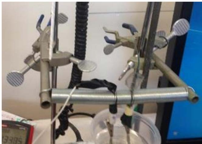
Figure 11. Stand Set-up to Suspend Samples above the Reactor Vessel
