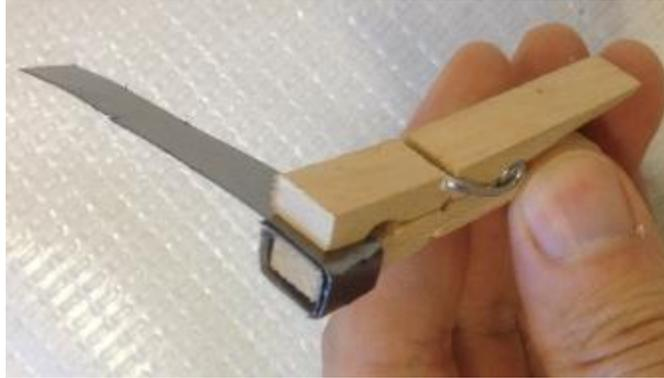
Figure 26. Modified Clothespin for Mounting the Anodized Sample
