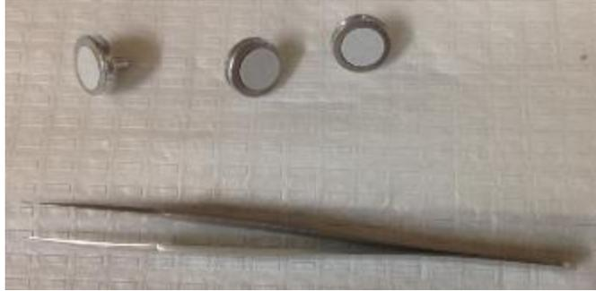
Figure 16. SEM Individual Sample Mounts with Attached Carbon Tape
