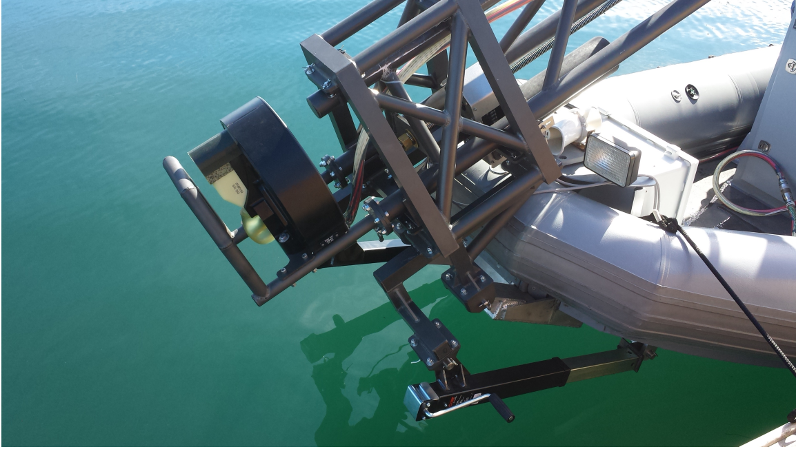
Figure 2.16. An ATLAS forward-looking sonar mounted on the NPS SeaFox USV.
