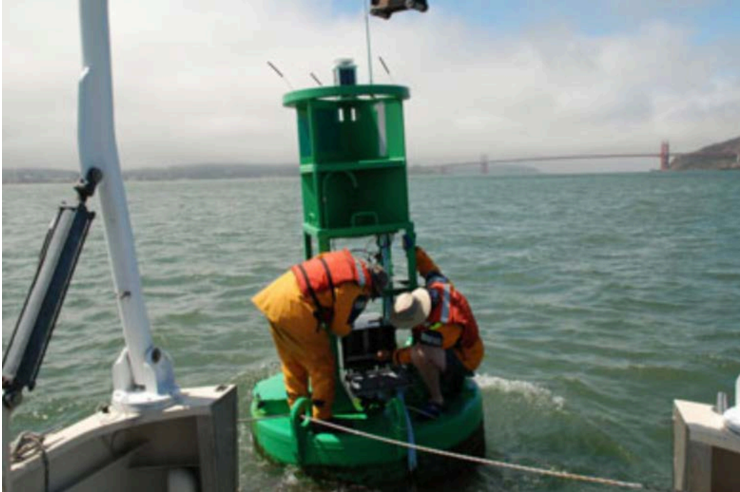
Figure 5. SEAWEB Gateway Installation on Coast Guard Buoy in San Francisco Bay. Source: [18].
