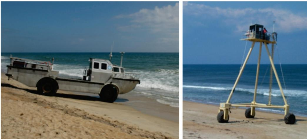
Because the surveys are used to quantify small changes in the nearshore profile, vertical accuracy has always been a concern and a major reason for using the CRAB, which allows an accurate land-based topographic survey
