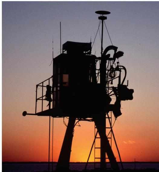
The most critical measurement to collecting accurate data with the CRAB is knowing the height of the GPS antenna above the ground. This is done by checking the elevation of a specific parking lot point during each day of surveying. During the survey test, the GPS antenna phase center to ground was measured with a plumb bob and recorded as 13.423 m.
