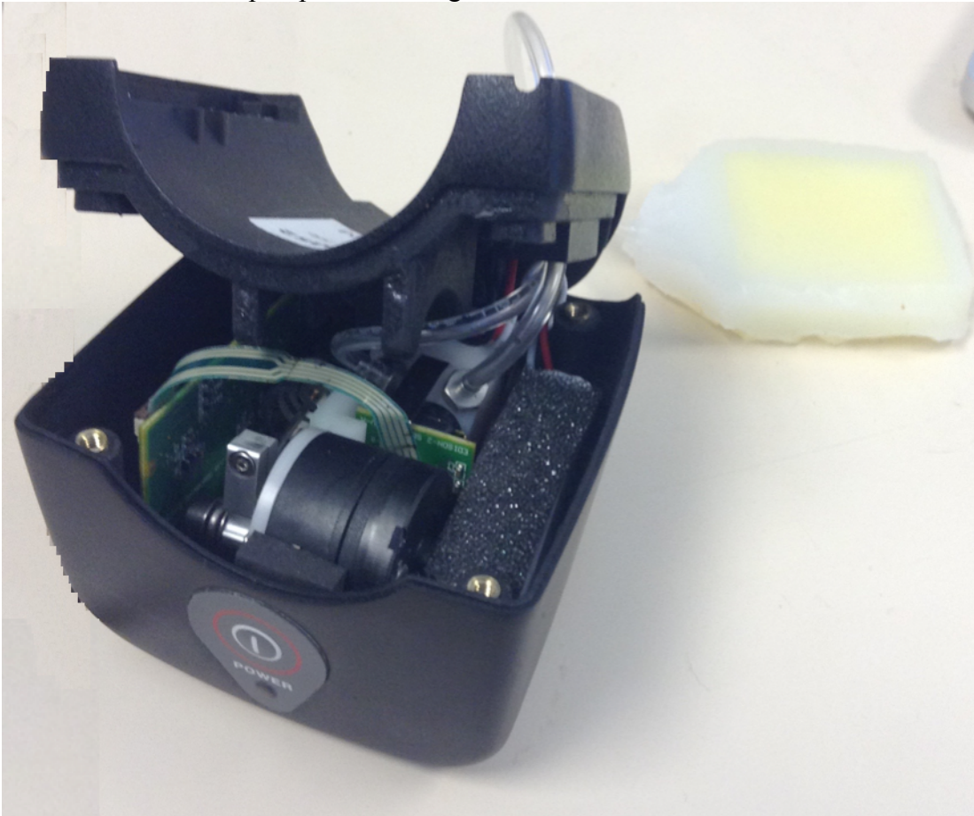
Figure 3 - The current vacuum pump design open so that the internal components are visible.
