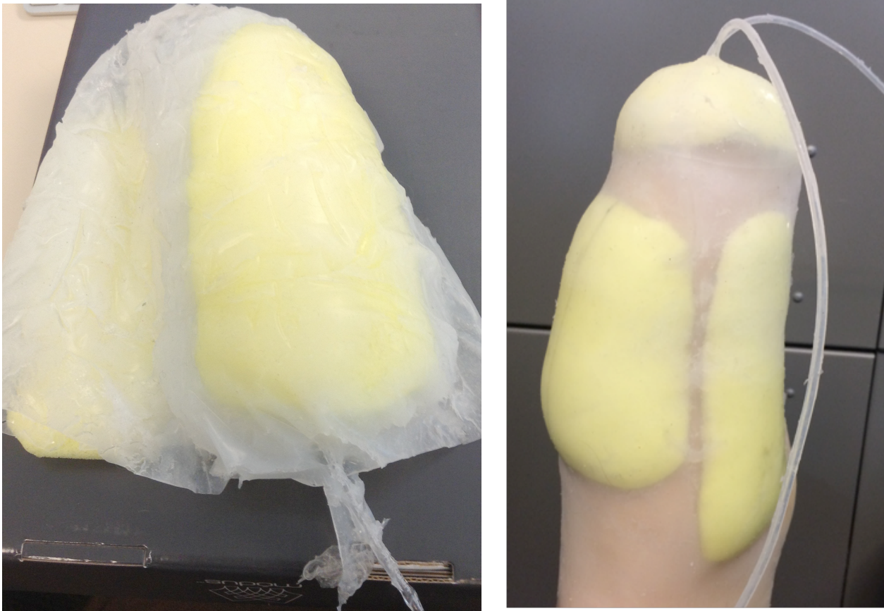
Figure 9 - Prototype liners investigating different manufacturing methods. Painted viscous silicon (left) and layering thin premade liners (right)
