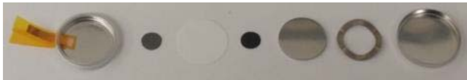
Figure 30. Coin cells with reference electrode (assembly order left to right)
