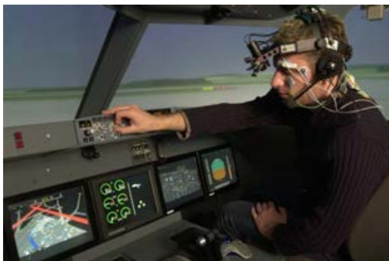
Figure 2. Subject equipped with iViewX (Sensomotoric Instruments) eye tracking system sitting in an Airbus style simulator (Biella, 2009)
