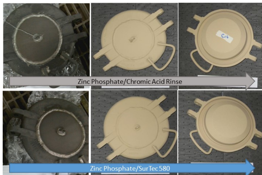
Figure 6-11. Phosphated, Sealed, Primed and Top-coated with CARC System at Anniston Army Depot
