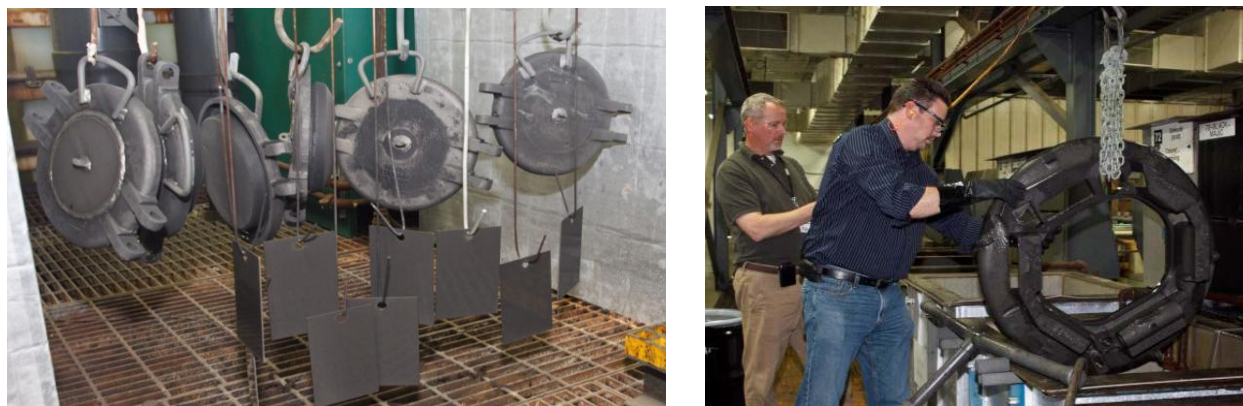
Figure 5-1. M1 Abrams Fuel Caps and Test Panels Zinc Phosphate and Sealed (left), Stryker Cupola Rising Out of the SurTec 580 Vat after Seal (right)
