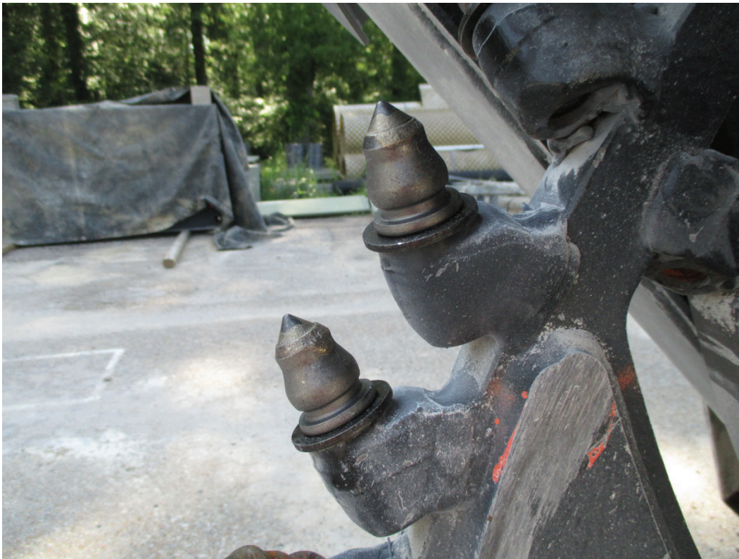
Figure 16. Prototype wheel saw tooth, Caterpillar 75148-1.
