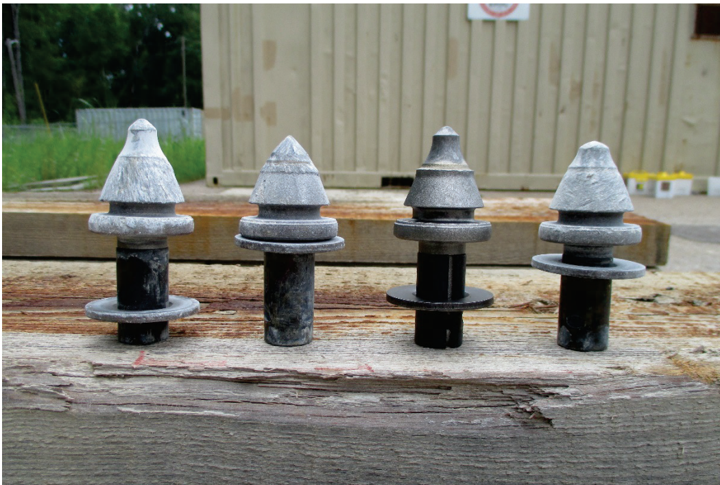
Figure 24. Inconsistent wear of Kennametal RP15 teeth on Caterpillar SW360B wheel saw.
