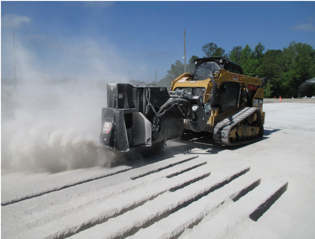
Figure 19. Caterpillar 299D XHP with SW460B wheel saw attachment.
