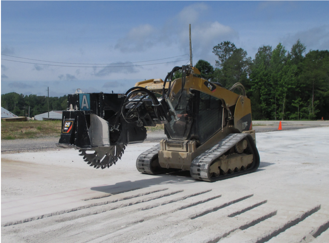
Figure 13. Caterpillar 279C CTL with SW45 wheel saw attachment.
