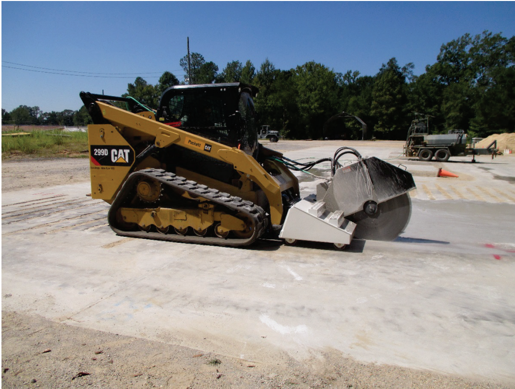
Figure 31. Caterpillar 299D XPS with SS4800HF attachment.
