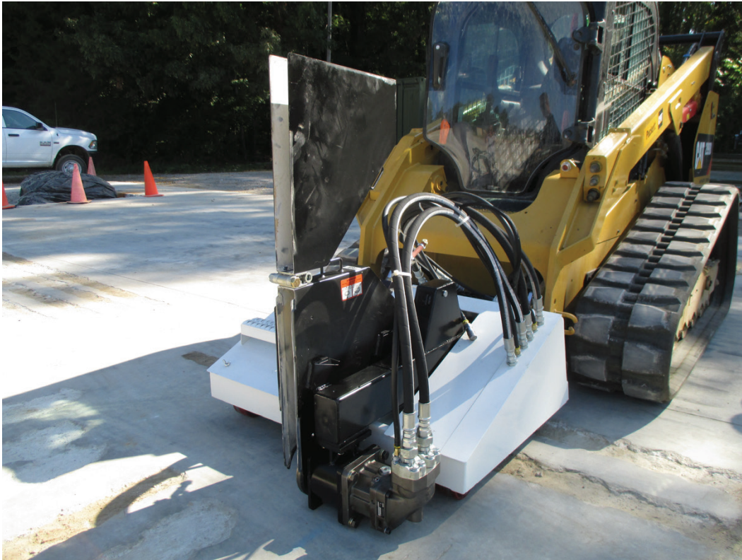
Figure 15. Cuts, Inc. SS4800HF diamond blade saw attachment without the blade.
