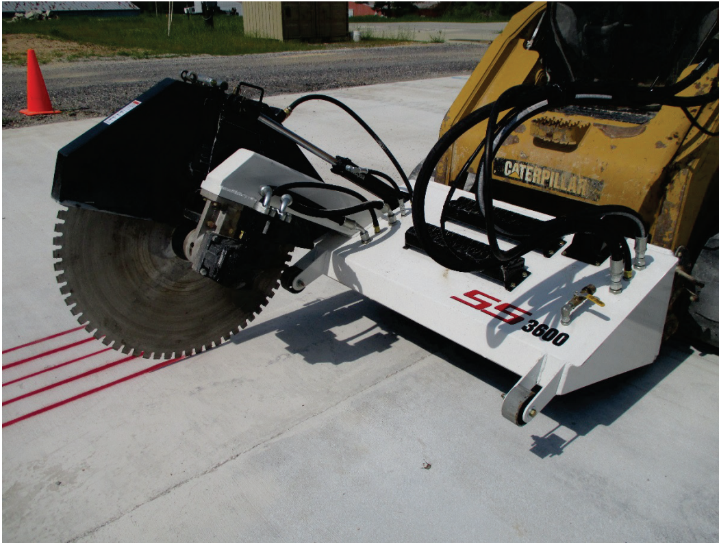
Figure 25. SS3600 diamond blade attachment mounted on a Caterpillar 279C XPS CTL.
