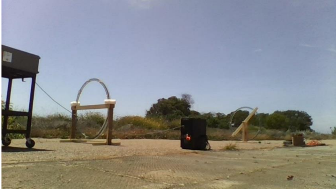
Figure 9. The two air loop antennas are supported by wood cradles. The WFS Technologies, Ltd. transceivers were placed on the ground (out of view). The UPS is the large black box near the middle of the photo and it powers the network analyzer (on a cart) on the left.
