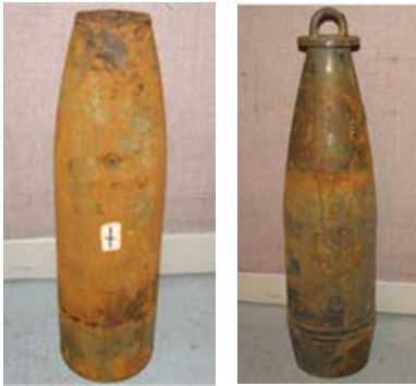
Figure 6. Shells after accelerated anodical polarization in a bath of 0.05M NaCl for a week simulating ~3 months of seawater exposure. (Left) 5 inch shell; (Right) 155mm shell.
