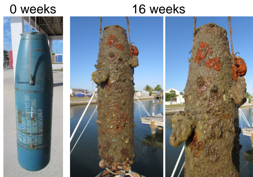
Figure 5. 5 inch shell: (left) clean shell; (center) after 16 weeks in biofouling site; (right) blow up of upper right.
