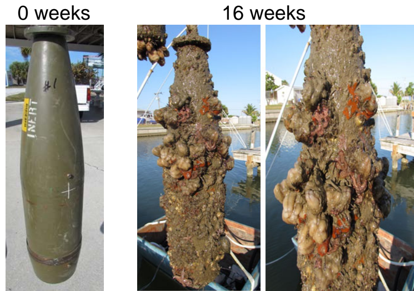
Figure 4. 155mm shell: (left) clean shell; (center) after 16 weeks in biofouling site; (right) blow up of upper right.
