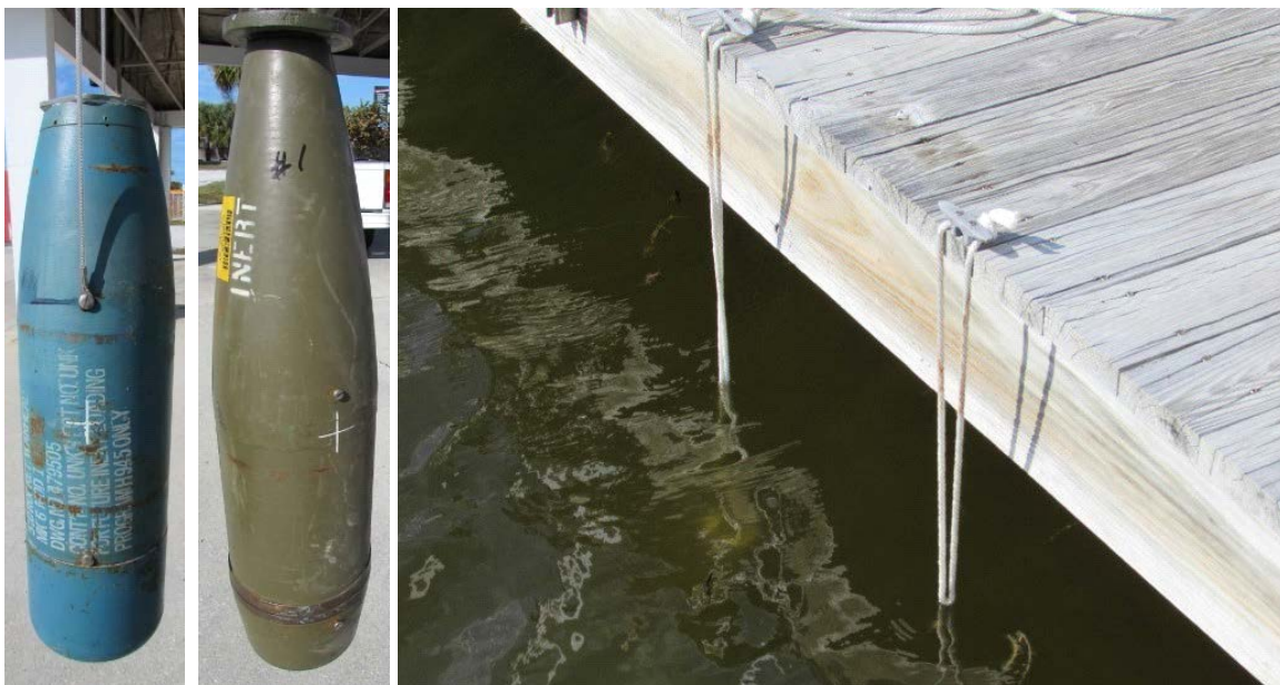
Figure 3. – (left) 155mm Howitzer shell, (center) 5-inch rocket, and (right) test setup on dock at Englewood, FL site.
