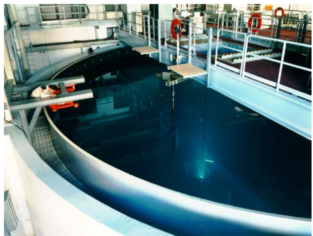
Figure 7. NRL 1M gallon structural acoustic pool facility.
