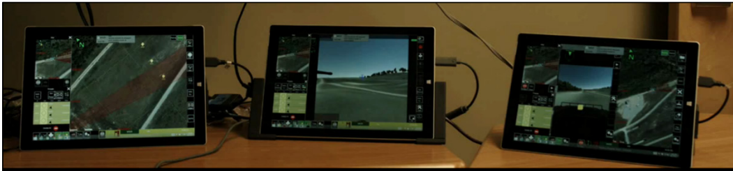
Fig. 8 Multiple WMI setup with Commander Display (left), Robotic Vehicle Gunner setup (center), and Robotic Vehicle Operator setup (right)
