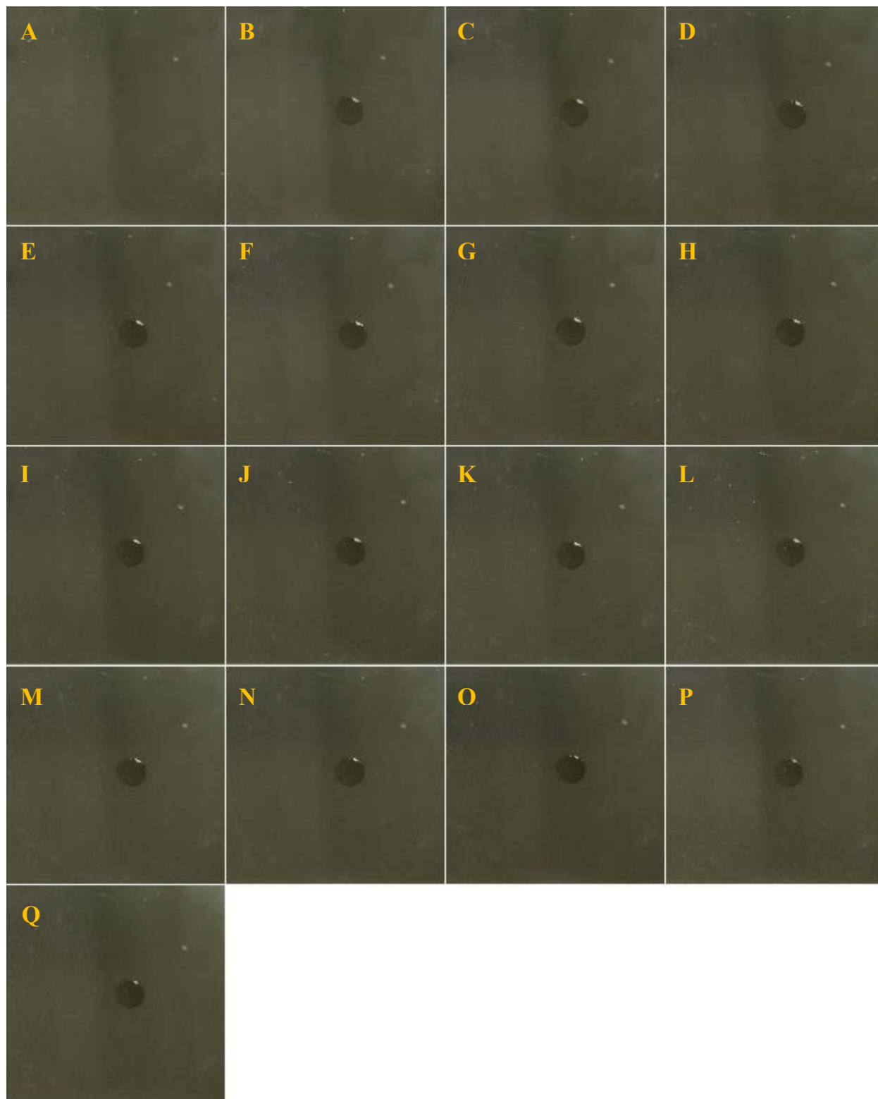
Fig. A16 — DFP on the SOCAL modified TEOS as synthesized surface. Images of a coupon before application (A) and at 0 (B), 0.5 (C), 1 (D), 1.5 (E), 2 (F), 2.5 (G), 3 (H), 3.5 (I), 4 (J), 4.5 (K), 5 (L), 10 (M), 15 (N), 20 (O), 25 (P), and 30 (Q) min following application of the target. These images were collected with a glass cover in place to limit evaporation. Reflections from the cover can be seen in some images.
