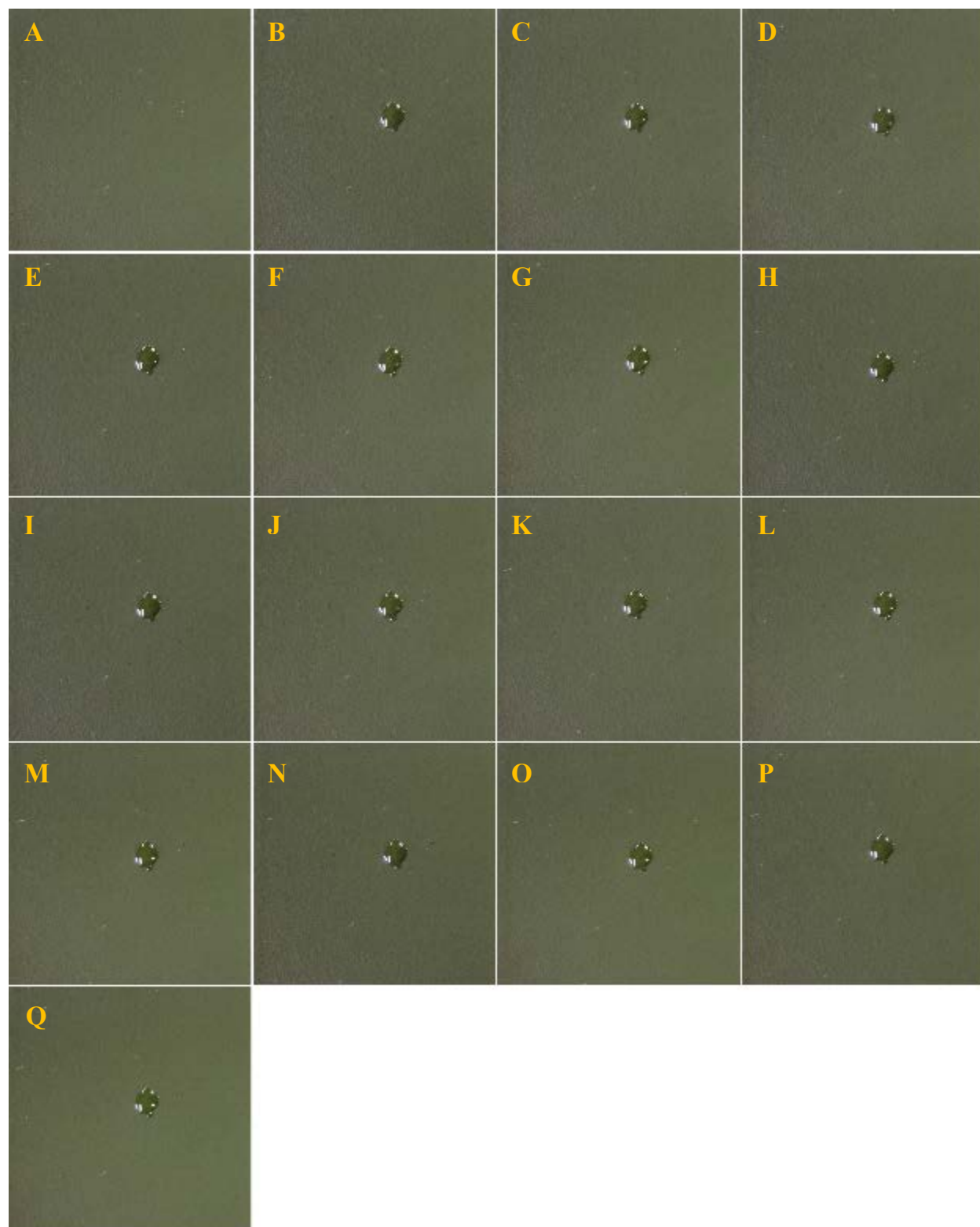
Fig. A18 — DMMP on the SOCAL modified TEOS as synthesized surface. Images of a coupon before application (A) and at 0 (B), 0.5 (C), 1 (D), 1.5 (E), 2 (F), 2.5 (G), 3 (H), 3.5 (I), 4 (J), 4.5 (K), 5 (L), 10 (M), 15 (N), 20 (O), 25 (P), and 30 (Q) min following application of the target.
