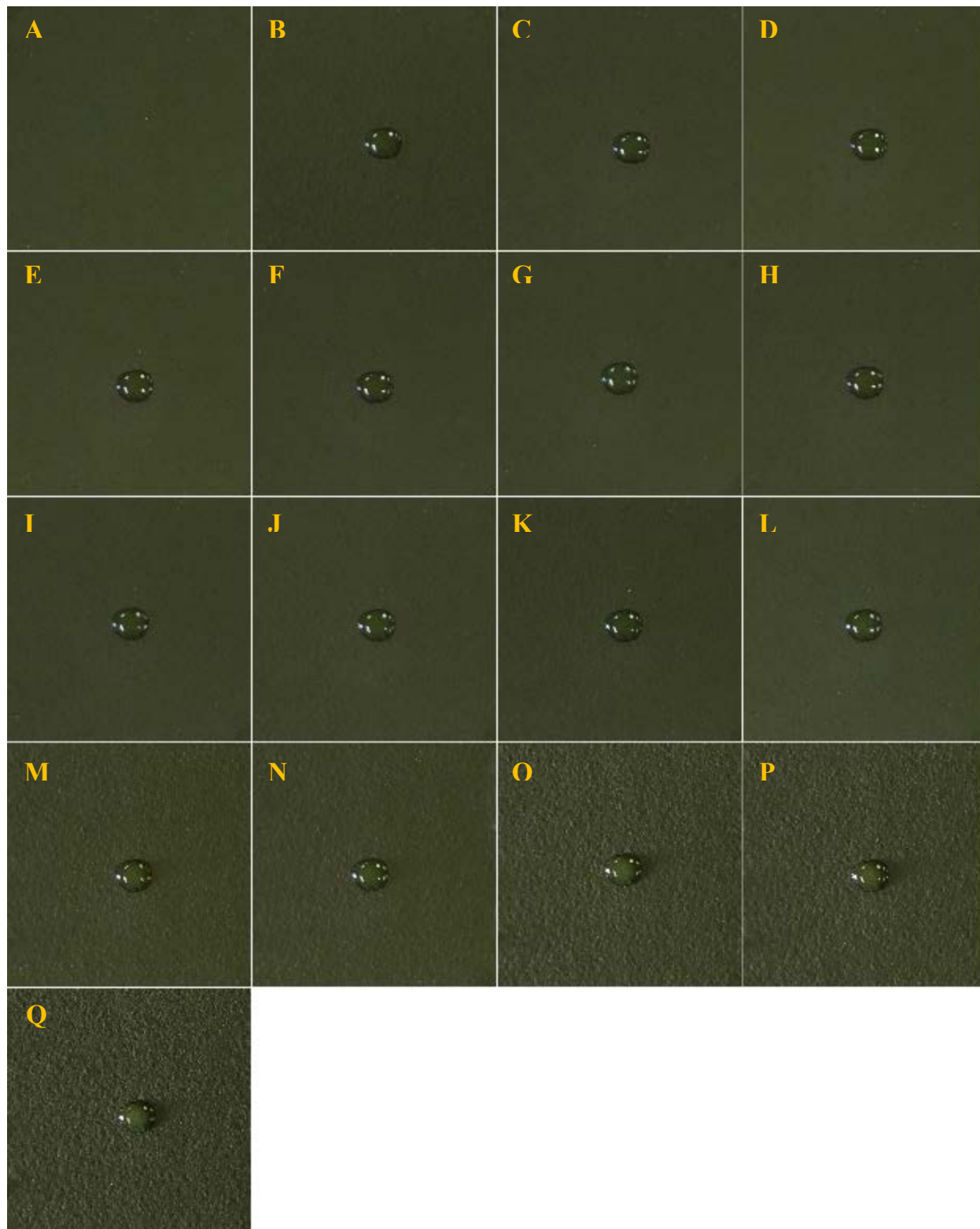
Fig. A12 — DMMP on the SOCAL modified ARSiO 2 extracted surface. Images of a coupon before application (A) and at 0 (B), 0.5 (C), 1 (D), 1.5 (E), 2 (F), 2.5 (G), 3 (H), 3.5 (I), 4 (J), 4.5 (K), 5 (L), 10 (M), 15 (N), 20 (O), 25 (P), and 30 (Q) min following application of the target.
