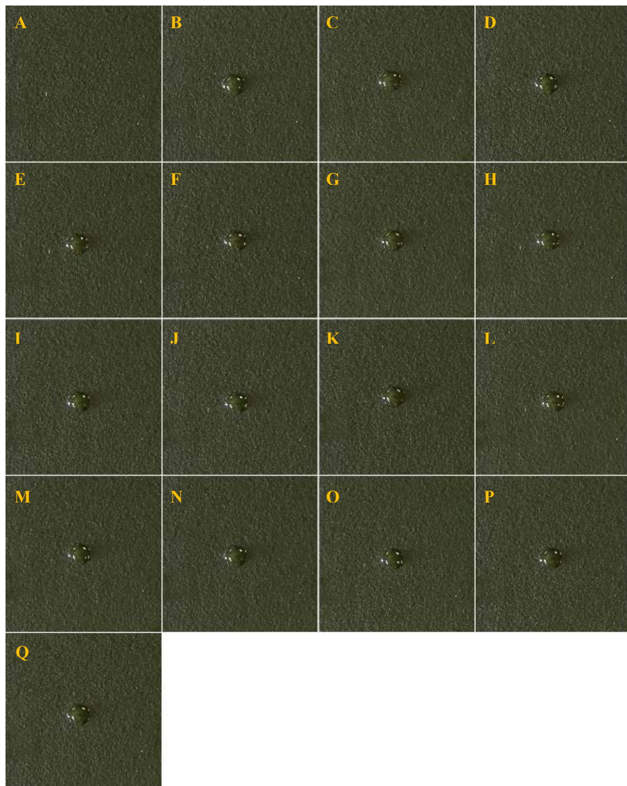
Fig. A11 — MES on the SOCAL modified ARSiO 2 as synthesized surface. Images of a coupon before application (A) and at 0 (B), 0.5 (C), 1 (D), 1.5 (E), 2 (F), 2.5 (G), 3 (H), 3.5 (I), 4 (J), 4.5 (K), 5 (L), 10 (M), 15 (N), 20 (O), 25 (P), and 30 (Q) min following application of the target.
