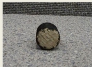
Figure 4. Top view of polymer electrode
