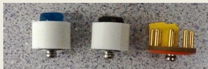
Figure 6. Side view of electrodes. From left to right: hydrodot, polymer, g.SAHARA
