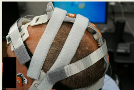
Figure 16. Side view of custom headset with electrodes snapped in
