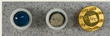
Figure 7. Top view of electrodes. From left to right: hydrodot, polymer, g.SAHARA
