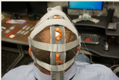
Figure 15. Posterior view of custom headset with electrodes snapped in
