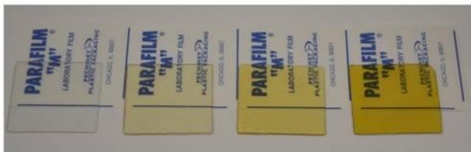
Figure 10. Plaques of PMMA blended with TR-PMMA, corresponding to 0% (I, left), 21% (III), 39% (IV), and 67% (VII, right) TR-PMMA.
