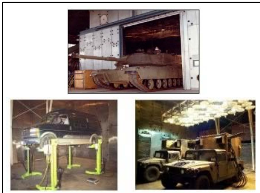
Figure 6. Multi-purpose Environmental Test Chamber.
