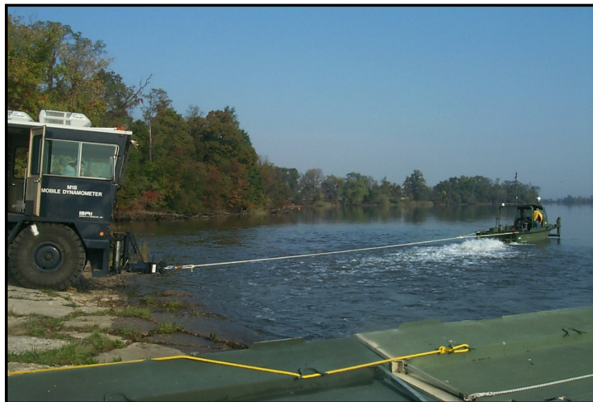
Figure 35. Bollard pull using mobile field dynamometer.
