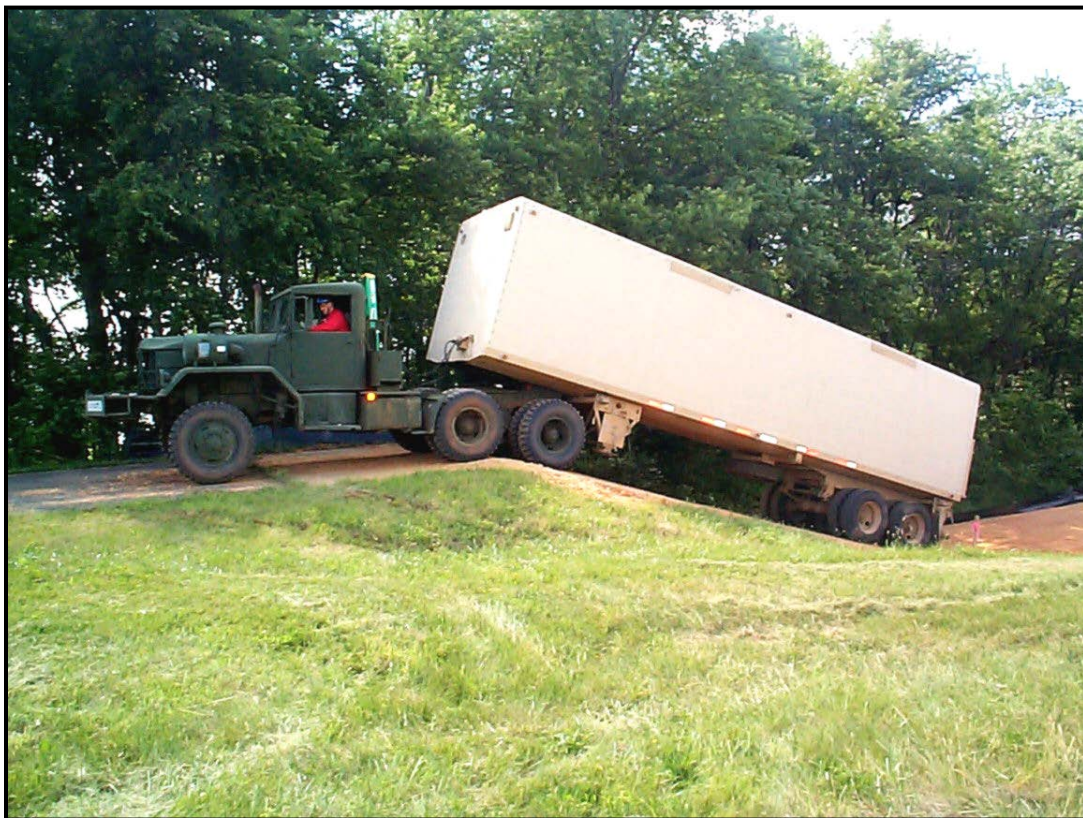
Figure 47. Vehicle on 20-degree simulated loading ramp.
