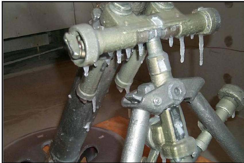
Figure 180. Test item after climatic icing test.
