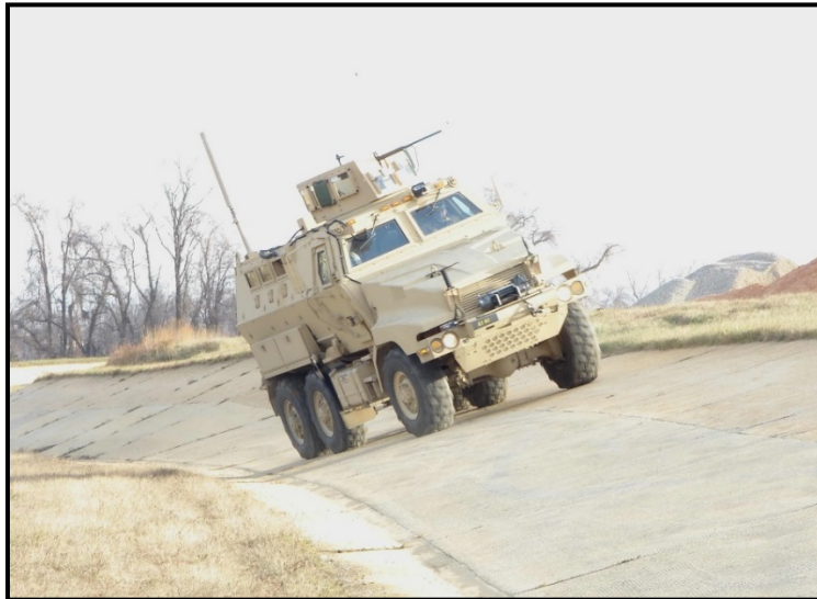
Figure 42. Vehicle negotiating the 20-percent side slope.
