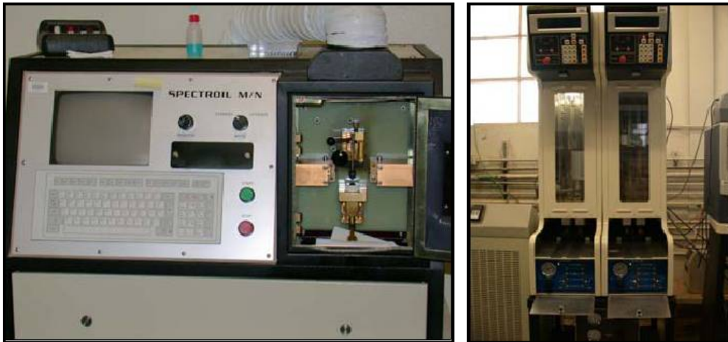
Figure 183. Spectroil rotating disk optical emission spectrometer used for wear metal analysis (left) and CAV2000 automatic viscometer used for measuring kinematic viscosity (right).
