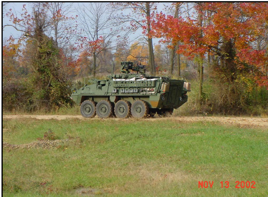
Figure 49. Testing wheeled vehicle suspension on 2-Inch Washboard Course.
