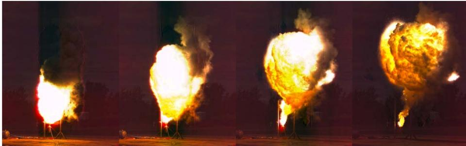
Fig. 9: Visible radiation from a flame propagating through a large-scale aluminium (12  $\mu\text{m}$  Valimet H-10 powder)-air dust cloud. Time between frames is 125 ms.
