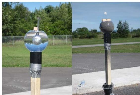
Fig. 2 Photographs of charges consisting of spherical glass casings containing either water (left) or iron powder (right). The C4 charge in the center of the sphere is visible in the charge on the left. The tube protruding from the C4 charge is used to insert the detonator into the C4.
