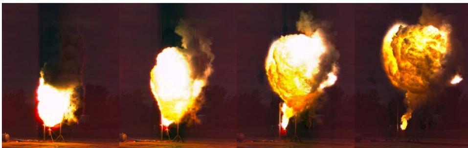
Figure 3. Visible radiation from a flame propagating through a large-scale aluminium (12  $\mu\text{m}$  Valimet H-10 powder)-air dust cloud. Time between frames is 125 ms.
