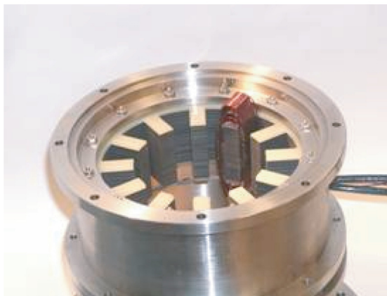
Figure 13.—Twelve-pole stator with one coil installed.
