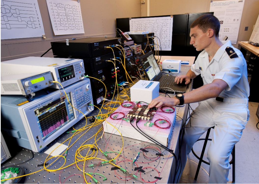
Fig. 5 Midshipman intern Drew Weninger operates the entangled photon distribution system in the ARL Quantum Network Testbed
