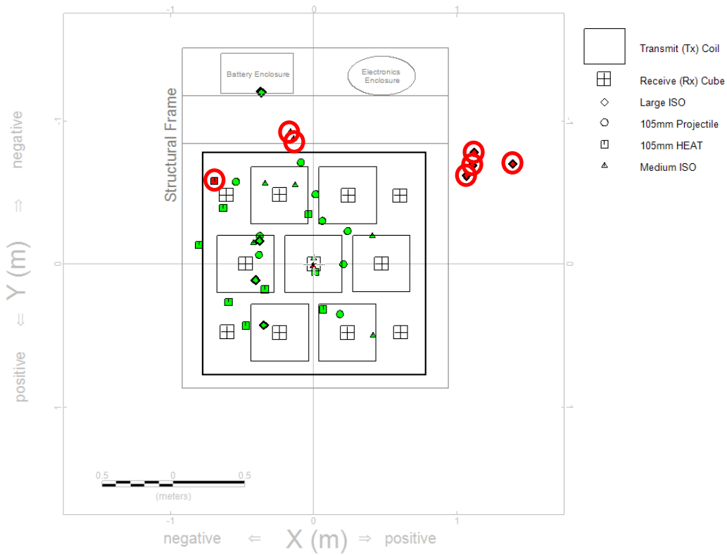
Figure 18. Buried target fit locations for ISOs and inert munitions. Green locations indicate >0.9 library match and red indicate <0.9. Circled locations indicate where the fit quality was good (>0.5) but the match to the corresponding library item was <0.9.
