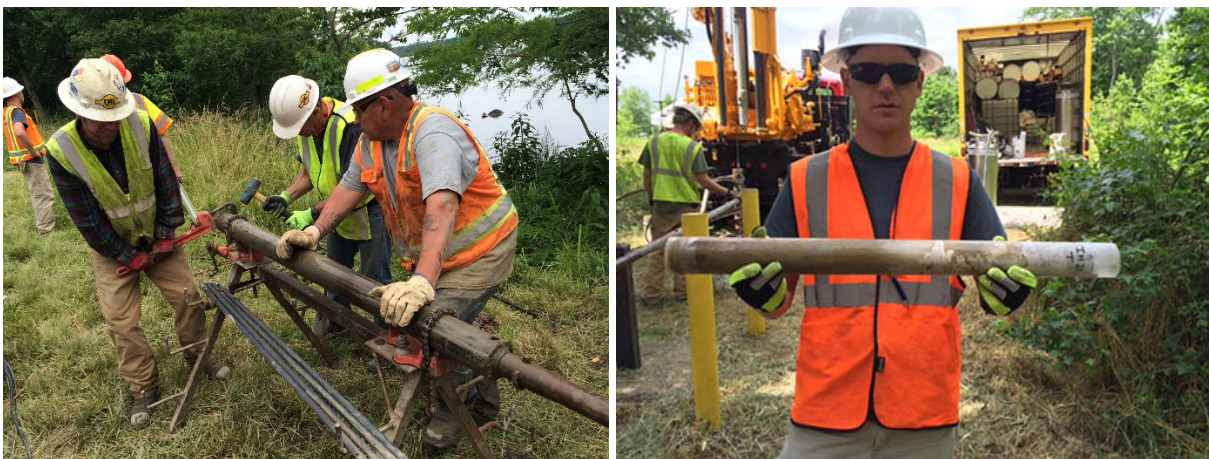
Figure 21. Photos of Frozen Core Removal from the Continuous Sampler.
