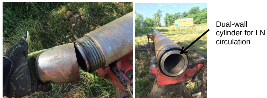
Figure 17. Photos of Core Barrel Sampler.
