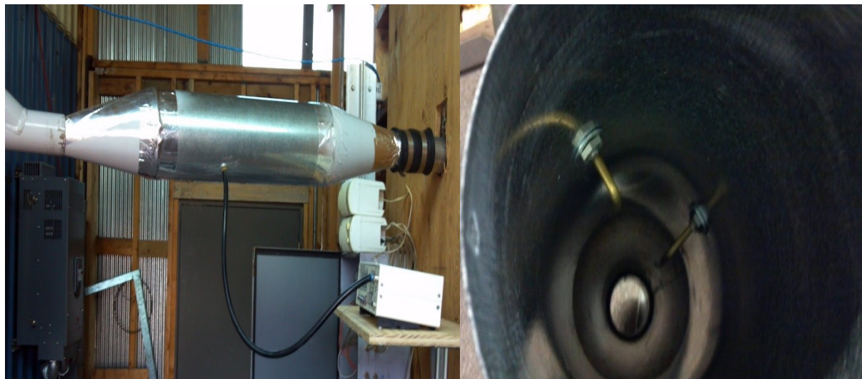
Figure A-9. Sub-sample expansion section inside (right) and outside view (left).
