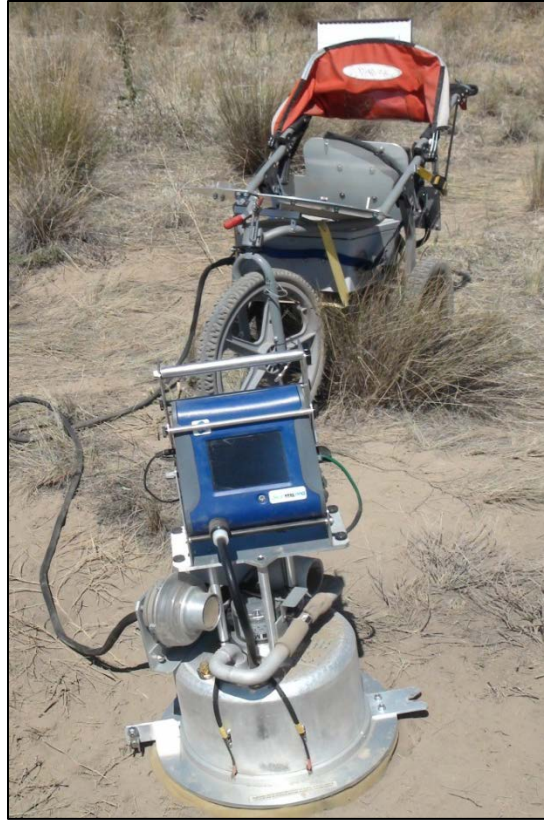
Figure 13. PI-SWERL setup in the field at Yakima Training Center, WA for collecting data.
