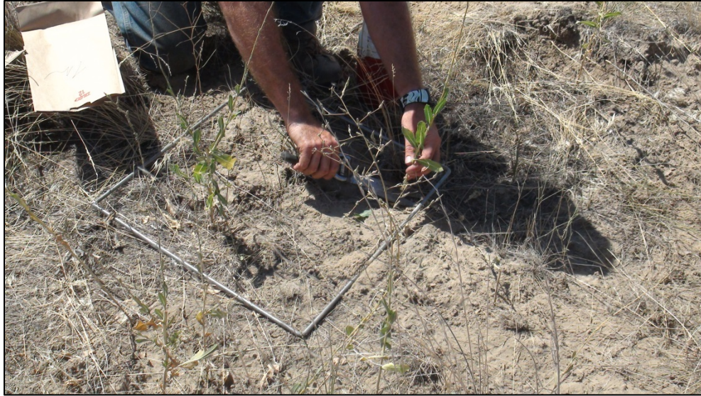
Figure 15. Soil attached biomass sampling method used at all sites.
