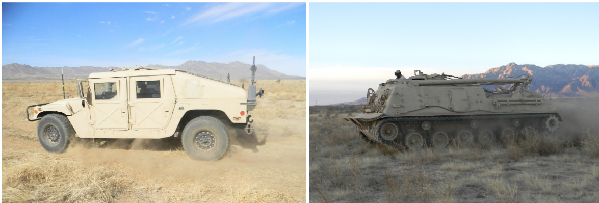
Figure 4. Up-armored HMMWV (left) and M88-A1 Tank Retriever (right) used at White Sands Missile Range, NM.
