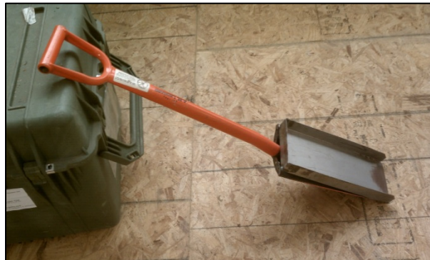
Figure A-2. Specially modified shovel for extracting wind tunnel tray samples.
