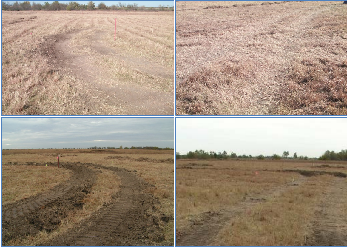
Figure 17. Figure-8 plot of curved traffic regions (left) and straight trafficked regions (right) for both the HMMWV (top) after 50 passes and the M1A1 tank (bottom) after one pass at Ft. Riley, KS.
