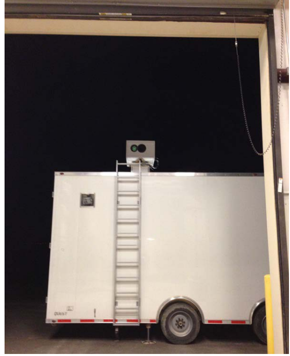
Figure 55. CELiS installed inside a Dugway Proving Ground test trailer and in position for use at the JABT. The left picture is the complete CELiS system placed on a hydraulic lift inside the trailer. The right picture is CELiS hoisted into position.
