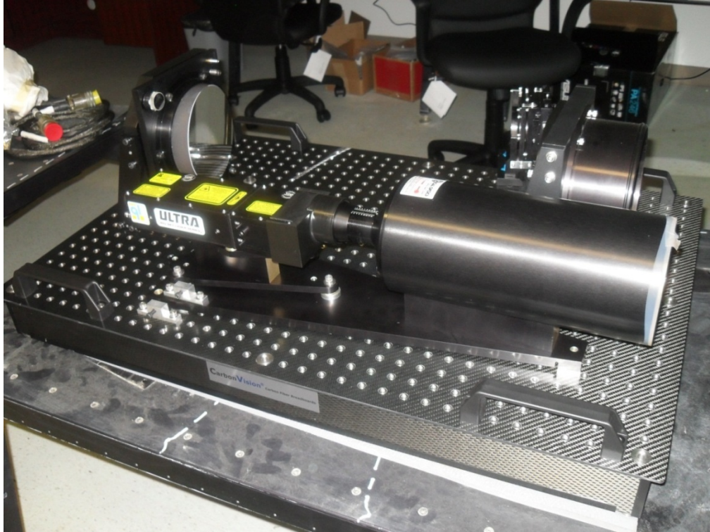
Figure B- 2. Two different views of the actual CELiS assembly. The optical breadboard is carbon fiber, chosen for light weight and low coefficient of thermal expansion.
