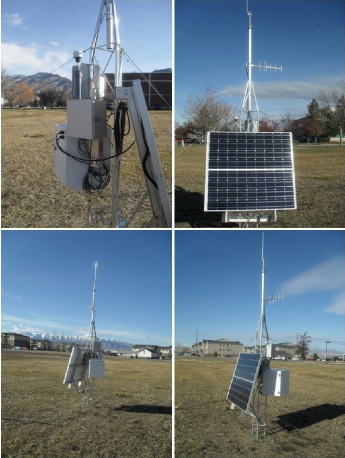
Figure B- 5. MetOne E-Sampler to be used for calibrating CELiS. E-Sampler subjected to 30 day trial run to assess its reliability.
