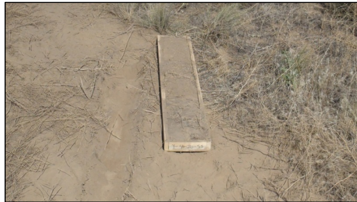
Figure 11. Wind tunnel tray sample extracted from the Yakima Training Center, WA site.
