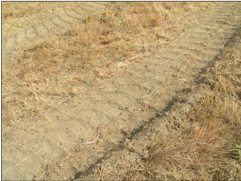
Figure 16. Beaded string method used for measuring surface cover at all sites.
