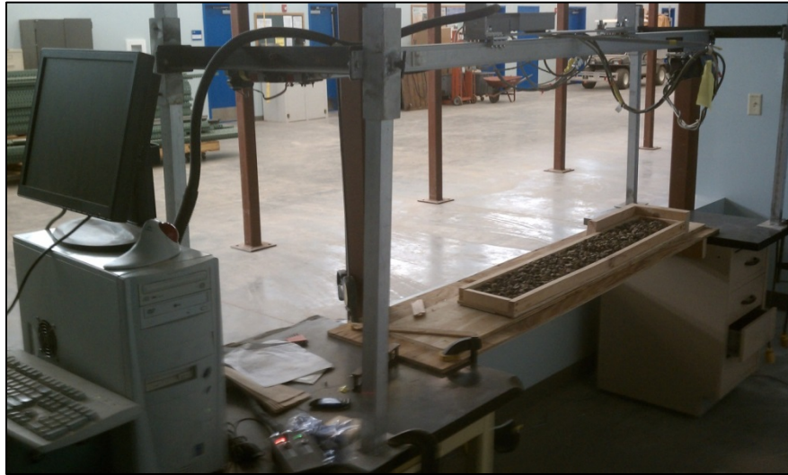
Figure A-7. Laser system used to scan surface roughness of wind tunnel trays.
