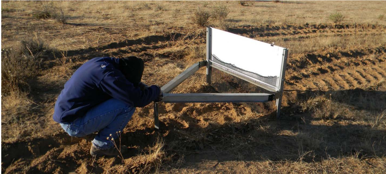
Figure 14. Using a pin meter to take transect surface elevation data across tracks at WSMR.
