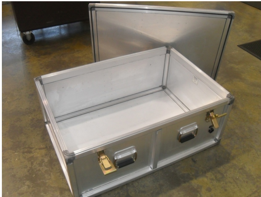
Figure B- 3. The hermetic enclosure for CELiS, prior to machining the penetrations for the cabling and the windows. The breadboard assembly drops directly inside this enclosure.
