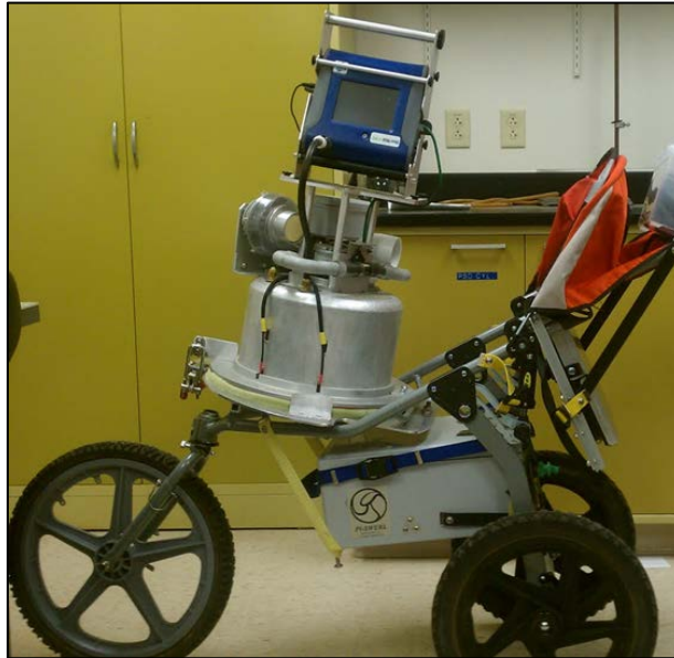
Figure 12. Portable In-Situ Wind Erosion Research Laboratory (PI-SWERL).
