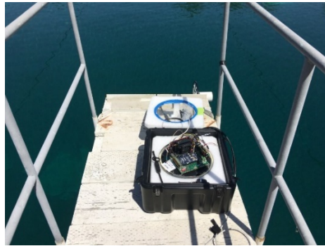
Figure 14. Photo showing modem hardware resting on deck at TRANSDEC.
