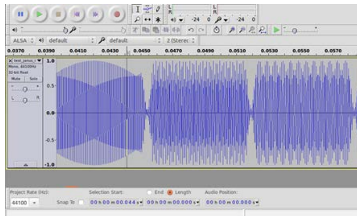
Figure 4. Time-trace containing JANUS signal generated by the transmitting modem.
