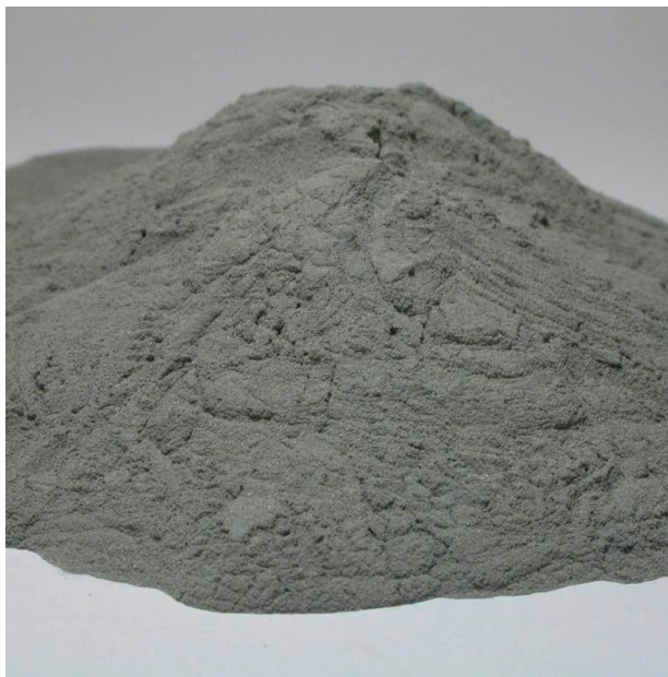
Figure 7.23 Fine aluminum powder (diameter \sim 20 \mu\text{m} ).
