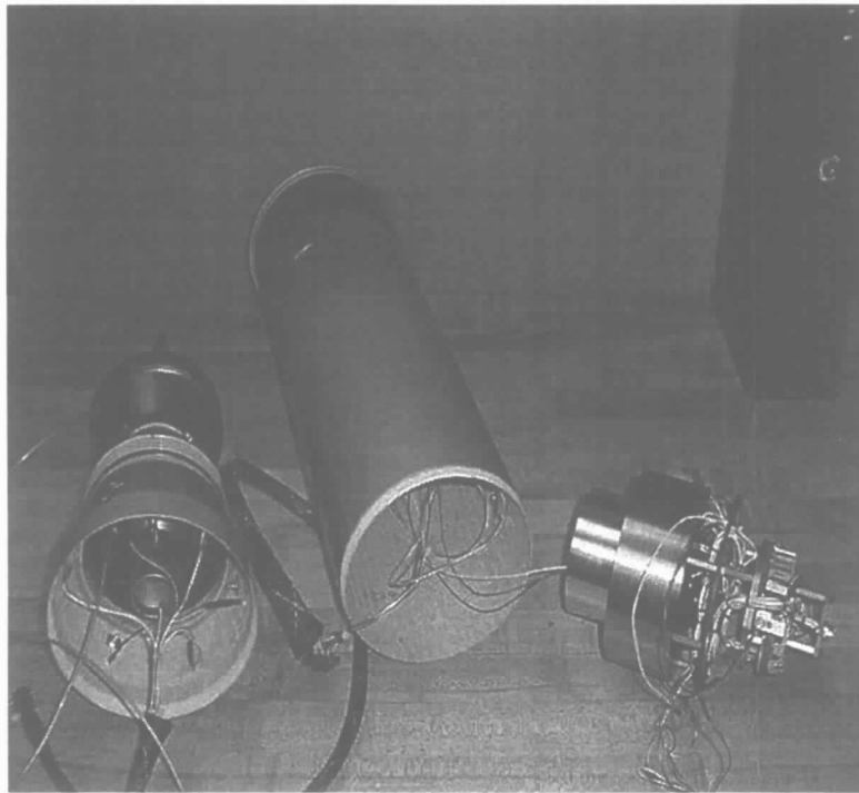
Figure 10 TM cartridge with projectile/case adapter and case base/cartridge case
