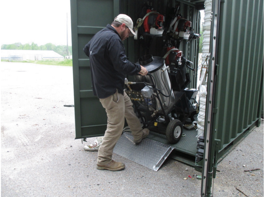
Figure 29. Unloading in-line water heater using metal ramp.
