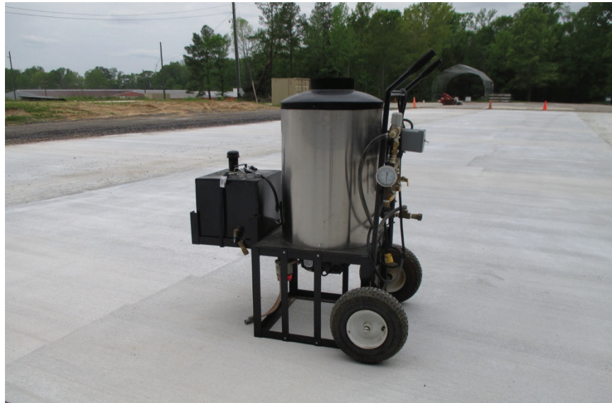
Figure 28. In-line water heater.
