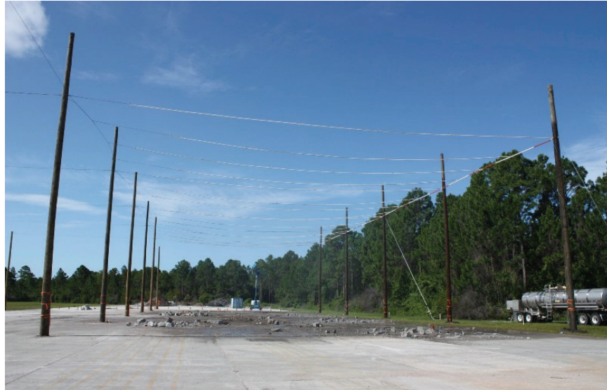
Figure 8. Calibrated sprinkler system used for wet weather crater repair tests.
