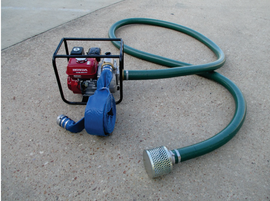
Figure 22. Water trash pump, discharge hose, suction hose, and strainer.
