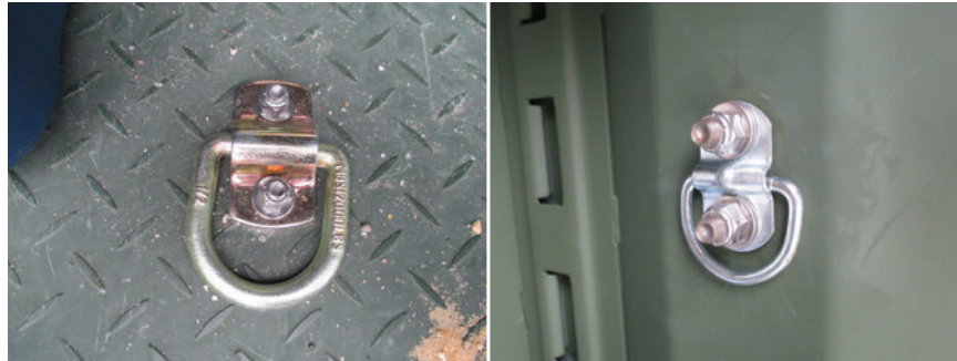
Figure 14. 12,000-lb (left) and 1,000-lb (right) surface mount rope rings.
