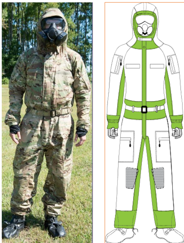
Figure 6 Picture of CBCC Type B prototype and concept sketch.
