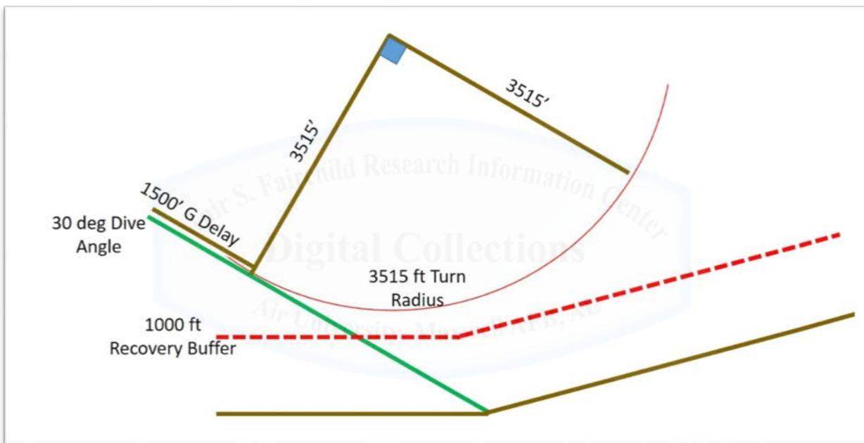
Figure 4. High-Angle strafe recovery (relationships to scale)
