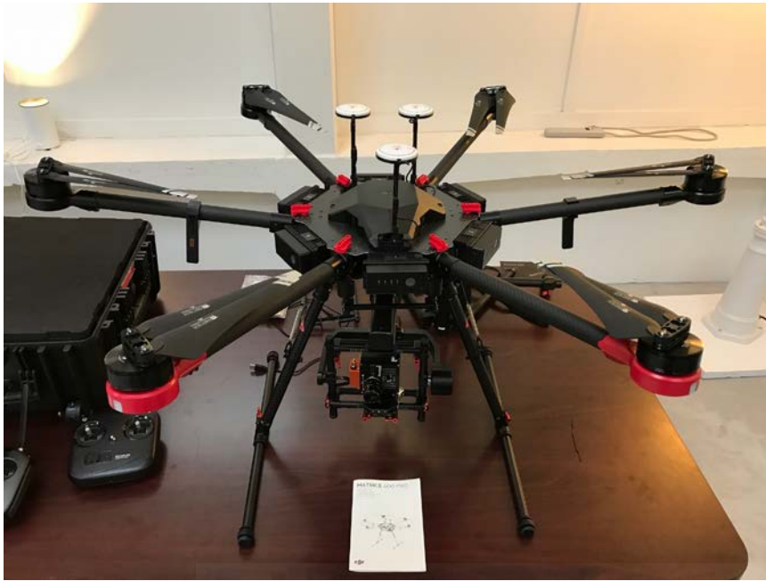
Figure 2: Headwall Photonics Nano-Hyperspec Integrated with DJI Matrice 600 sUAS 18
