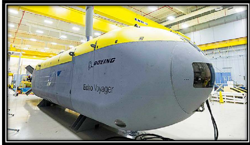
Figure 4. Boeing's Unmanned Undersea Cargo Vehicle, "Echo Voyager." 22
