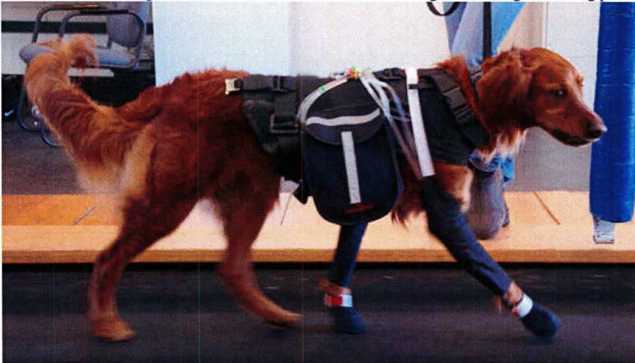
Figure 7: Photograph of a dog performing treadmill exercise with the initial prototype of the canine footpad cooling device.
