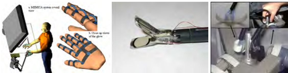
Figure 2: (left) Electro-rheological fluid (ERF) based haptic surgeon hand interface (Bar-Cohen et al., 2001); (center) Force transducer fitted to endoscopic grasper; (right) Pneumatic haptic finger tip display (Culjat et al., 2008) integrated with da Vinci ® hand controllers.
