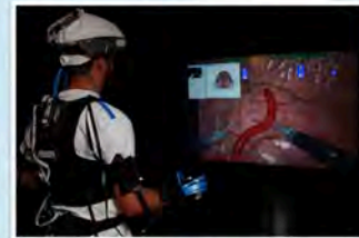
Figure 3: ACMI-SATS in software robotic surgical simulation (dv-trainer, mimic Technologies, Inc., Seattle, WA) demonstrating head and full body motion capture integrated with auditory and tactile information displays (inset shows graphical representation of manipulator shafts and grasper angle; each also indicates the forces on the end effectors).
