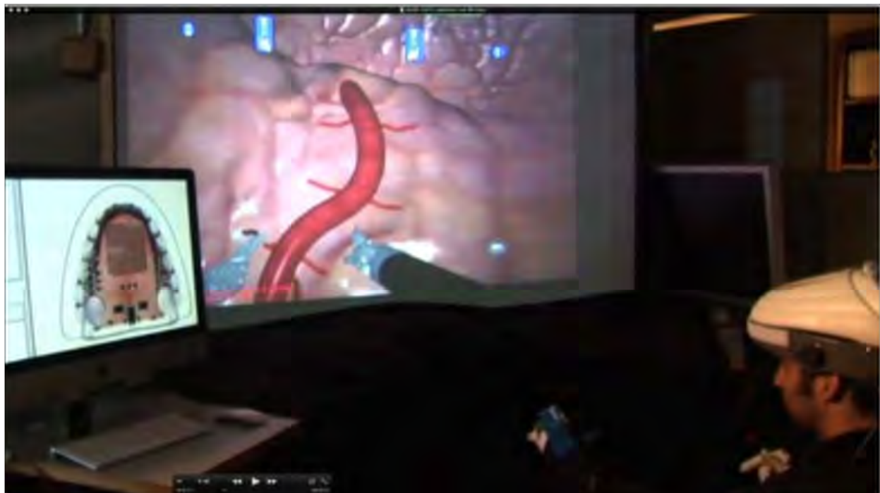
Figure 9: Mimic dV-Trainer imagery projected a reasonable approximation of the size of the human hand and arm. Motion capture of hand and arm movements maps 1:1 to onscreen robot movement. This allows for veridical kinesthetic and proprioceptive cues to augment visual information. Screen on left shows graphical representation of electrotactile stimulus on the tongue that represents closure angle (distance between tactile icons) and forces (intensity of stimulus) on the two (right and left) grasper end effectors.
