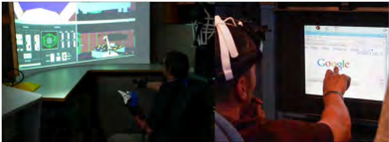
Figure 6: (left) Gesture based controller for robotic arm simulator. (right) Status post binocular enucleation, a servicemember uses his prosthetic eyes to control a tracking reticle on the screen with tactile (tongue based) display of area displayed inside the reticle (near user's finger).
