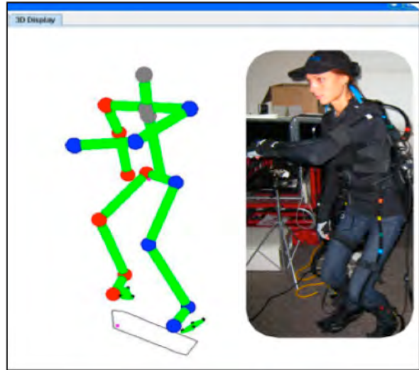
Figure 5: Body position (inset) tracked with ShapeWrap system using IHMC's AMI architecture. Box projected under avatar indicates stable platform for a given stance.
