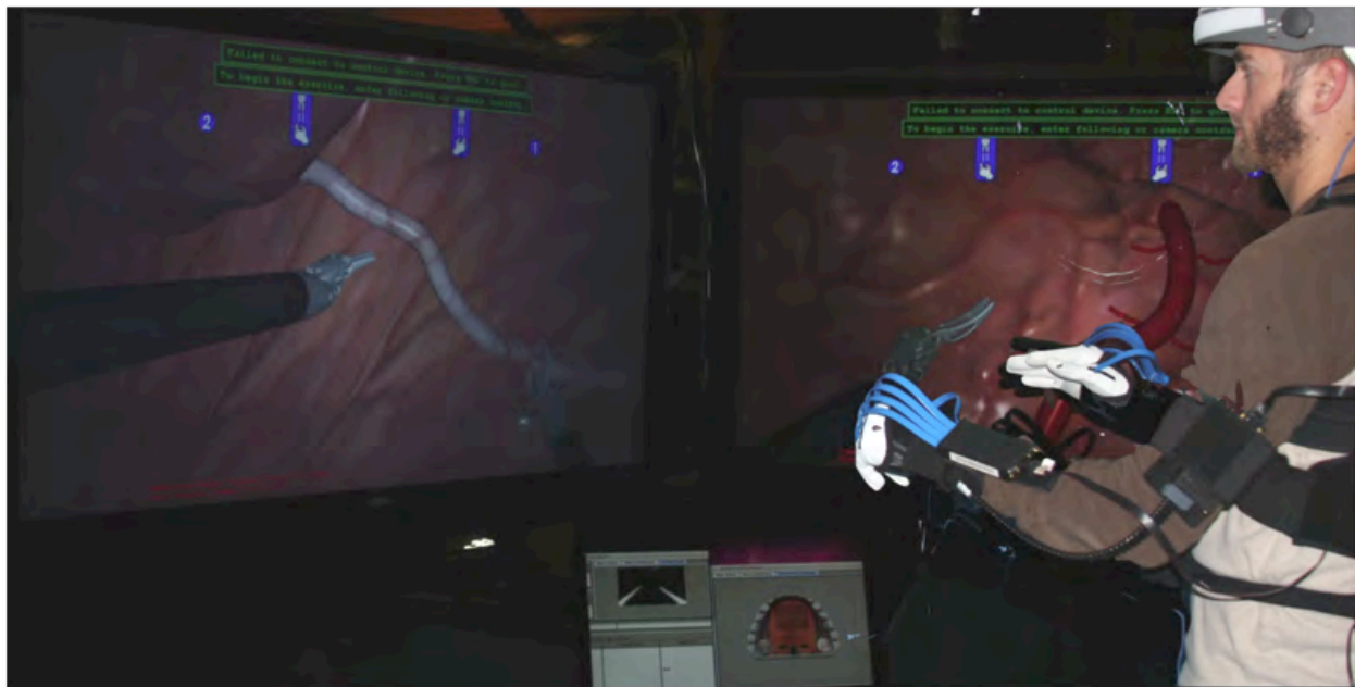
Figure 17: ACMI-SATS implementation with Mimic dV-Trainer showing single surgeon management of two simultaneous cases. The end effectors and camera view move with the user in one case at a time, selected by intuitive user gestures. Tactile interfaces (lower center) provide sensory augmentation for the currently active case by providing position and force information to the user.
