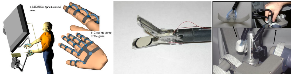
Figure 2: (left) Electro-rheological fluid (ERF) based haptic surgeon hand interface (Bar-Cohen et al., 2001); (center) Force transducer fitted to endoscopic grasper; (right) Pneumatic haptic finger tip display (Culjat et al., 2008) integrated with da Vinci ® hand controllers.
