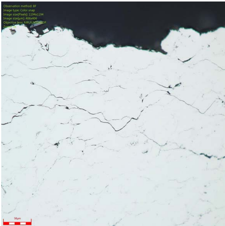
Figure 8 Higher magnification micrograph of cold sprayed 316 stainless steel powder (-325 mesh) made by Molyworks. Prevalent microcracking can be seen.
