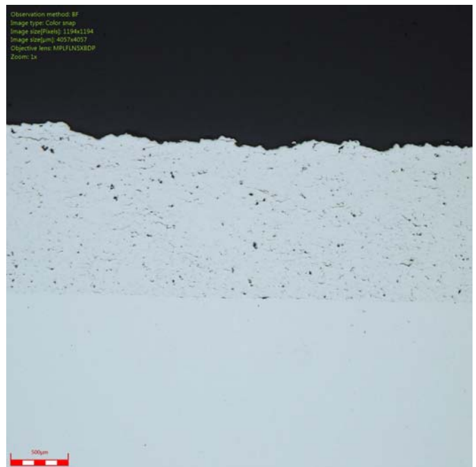
Figure 6 Micrographs of cold sprayed 316 stainless steel powder (-325 mesh) made by Praxair (left) and the Molyworks mobile foundry (right). Although the Molyworks deposit appeared to have less porosity, it contained microcracking.
