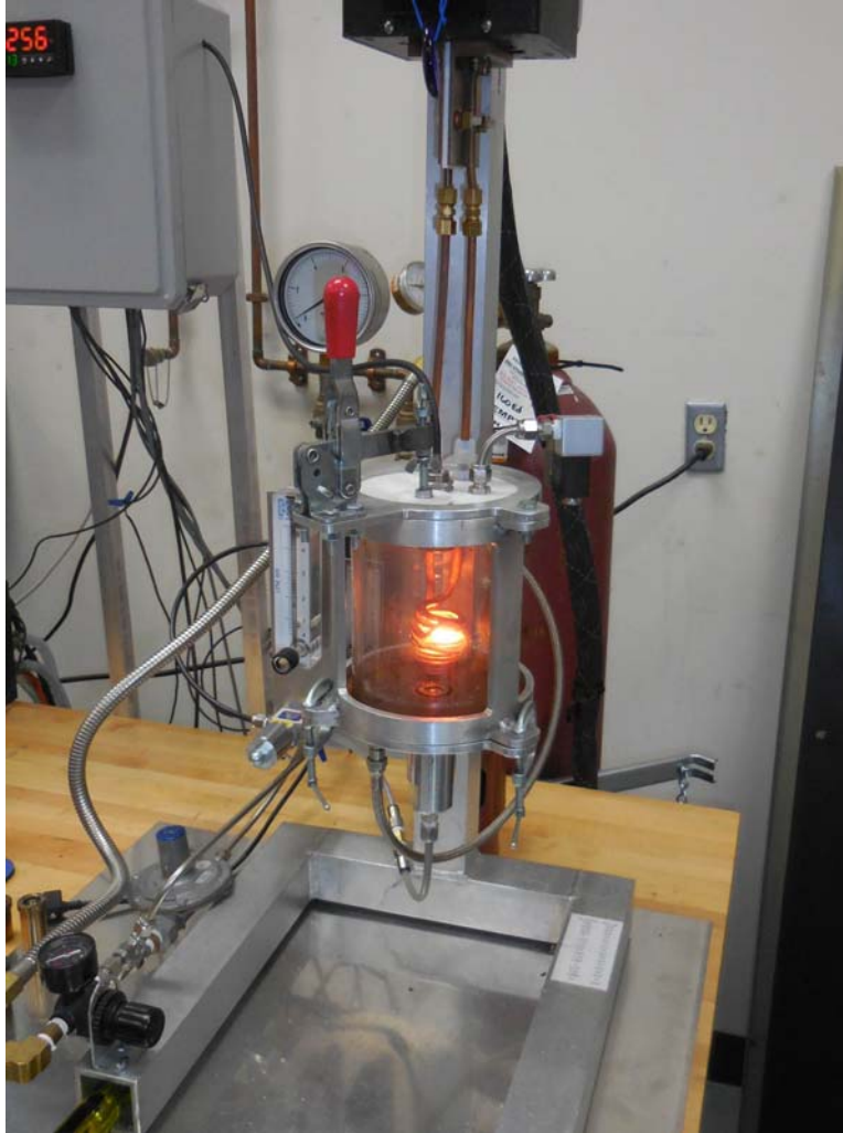
Figure 1 Lorenz force projection and melting technique proposed by AEM for production of AM-grade metallic powder on the battlefield.
