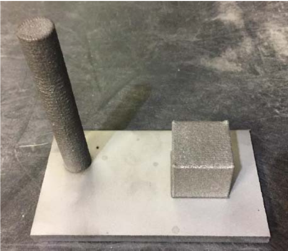
Figure 11 Tensile rod and cube built from 316 SS powder made in the mobile foundry using LENS technology.
